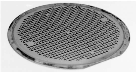
Fig. 4. Photograph of microdiaphragms fabricated on a 5-inch Si wafer.
