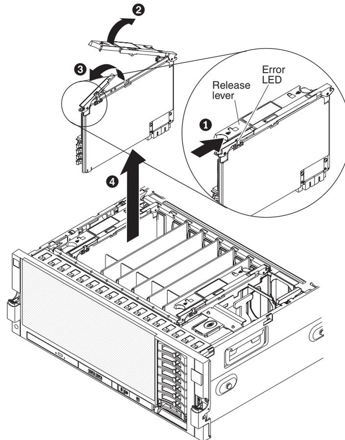
4. If you are installing DIMMs in a memory card that is already installed in the server, remove the memory card:
