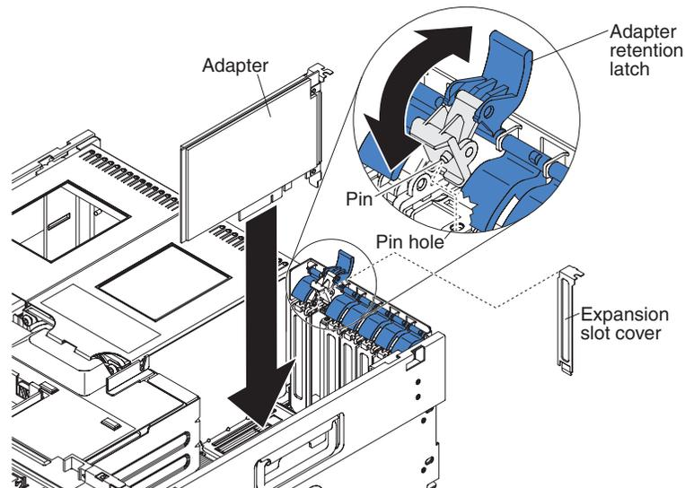
5. Push the adapter retention latch toward the rear of the server and open the tab.
