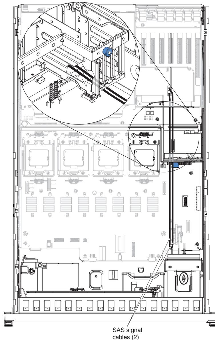
12. Connect one end of each SAS signal cable that came with the eXFlash drive cage and backplane option to the backplane and the other end to the ServeRAID adapter.
