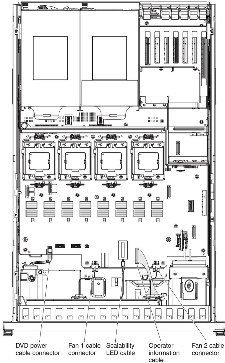
The following illustration shows the routing of the USB and DVD signal cables.
