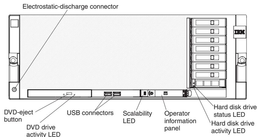
**Electrostatic-discharge connector:** Connect an electrostatic-discharge wrist strap to this connector when you work with static-sensitive devices.
