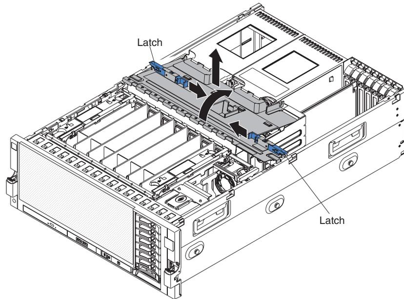
6. Tilt and lift the top-cover bracket out of the server.
