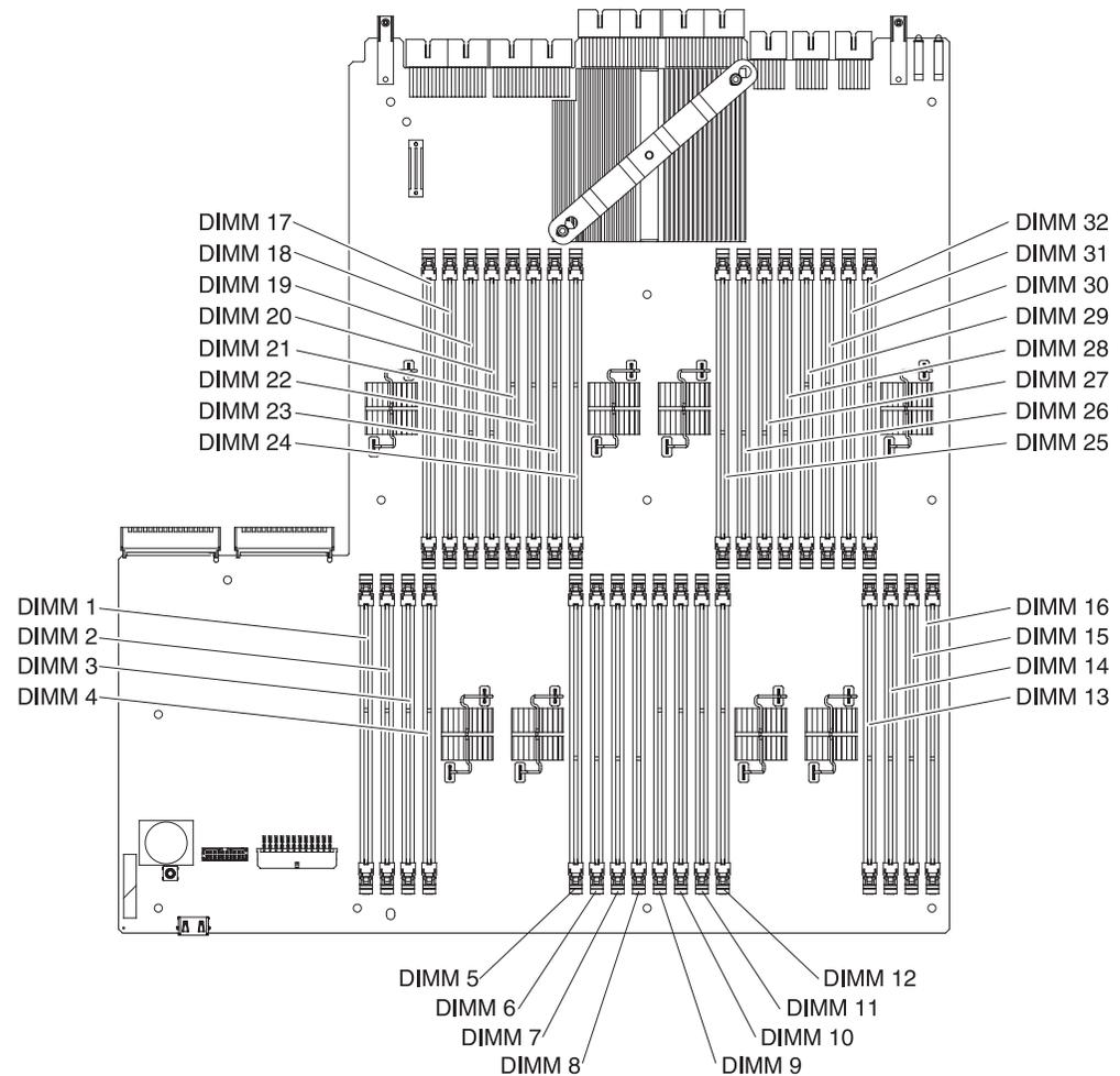
To install a DIMM (memory module) in the memory expansion module, complete the following steps.
