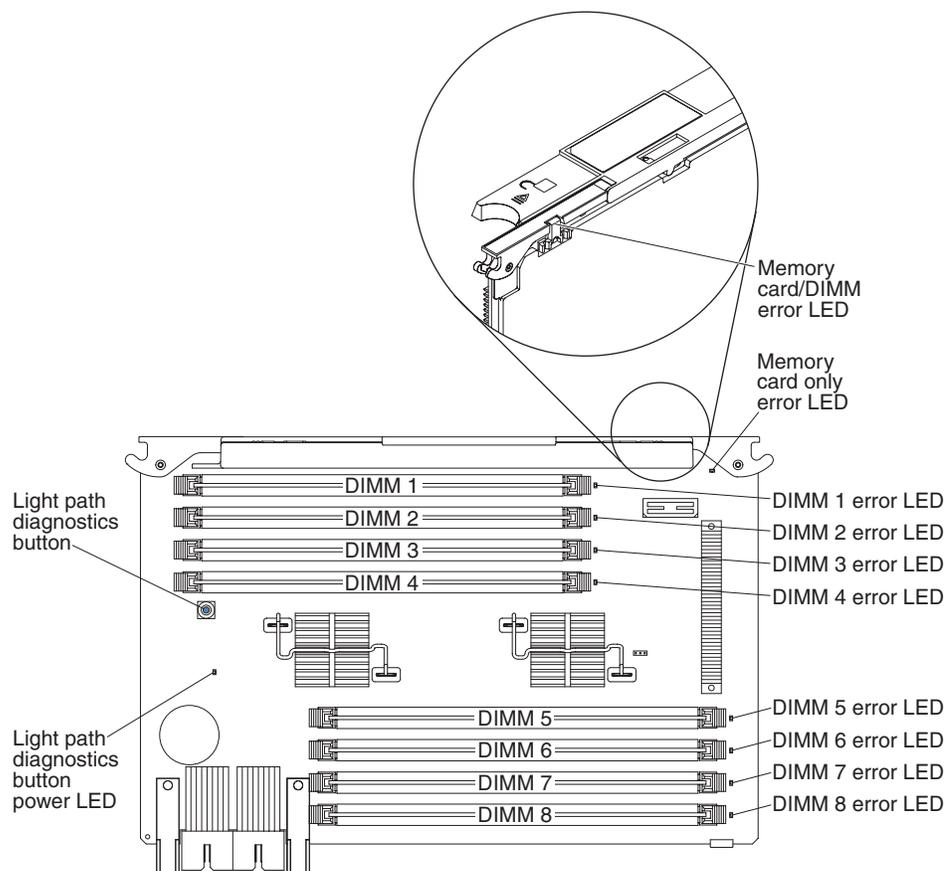
**Memory card/DIMM error LED:** When this LED is lit, it indicates that the memory card or a DIMM has failed.
