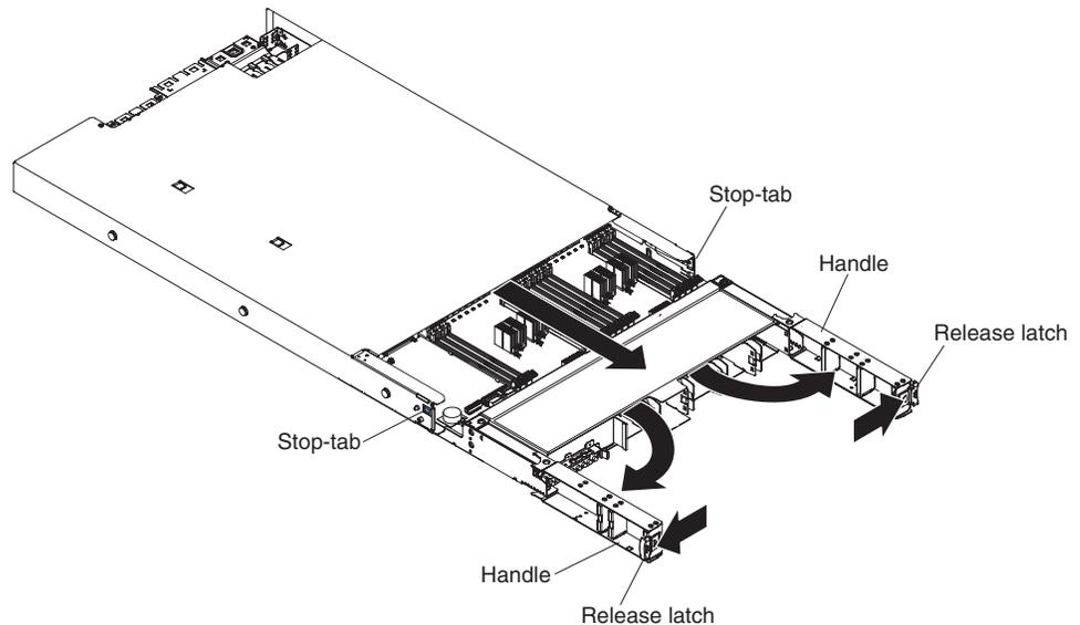
3. Slide the system-board tray forward until the tabs at the bottom of the handles touch the chassis; then, close the handles and press firmly on the release latches to snap them into the locked position.
