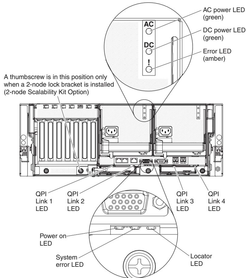
**AC power LED:** Each hot-swap power supply has an ac power LED and a dc power LED. When the ac power LED is lit, it indicates that sufficient power is coming into the power supply through the power cord. During typical operation, both the ac and dc power LEDs are lit. For any other combination of LEDs, see the *Problem Determination and Service Guide*.
