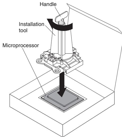
10. Carefully position the microprocessor with the microprocessor tool over the microprocessor socket. Twist the microprocessor tool counterclockwise to insert the microprocessor into the socket.
