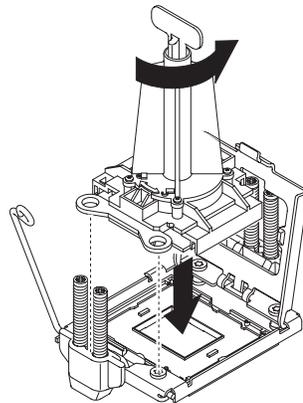
11. Close the load plate and then rotate the microprocessor-release lever to secure the microprocessor.
