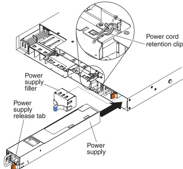
6. Route the power cord through the power cord retention clip so that it does not accidentally become disconnected.
