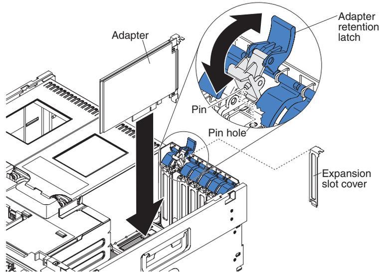
6. Remove the expansion-slot cover.
