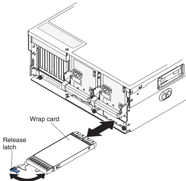
In a one node server only, if your server has more than two microprocessors installed, you must install two QPI wrap cards in the server.
