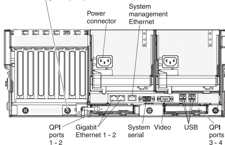
**Power-cord connector:** Connect the power cord to this connector.
