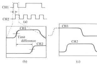
This means that CH1 is used as the triggering signal when investigating the length of time by which the signal of CH2 is delayed from the signal of CH1. CH2 is used in the reversed case. In other words, the signal leading in phase is selected as the triggering signal source.
