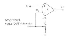
Fig. 7–1 Diagram of DC OFFSET
