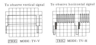
(NOTE) This oscilloscope synchronizes with only (-) synchronizing signal.
