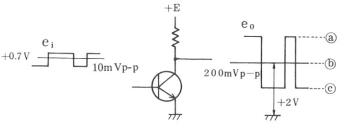
Fig. 7–2 Transistor amplifier
