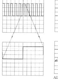
ALT MAG function (x1 waveform and x10 waveform)
