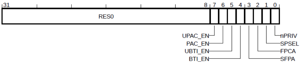
Figure 5-7: The CONTROL register
