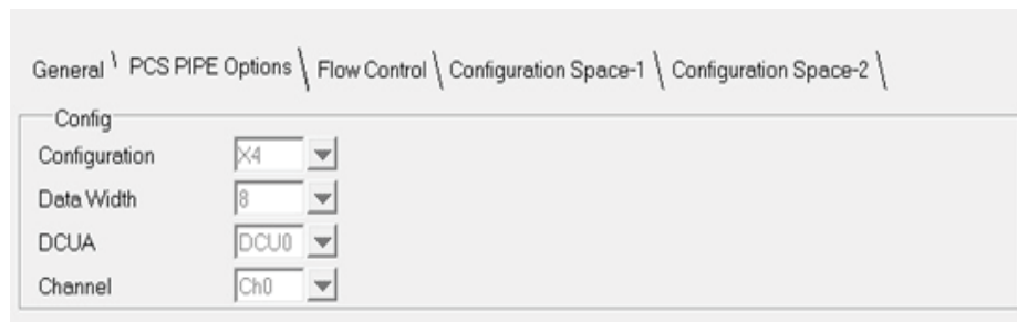
Figure 3.2. PCI Express IP Core PCS Pipe Options
