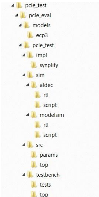
Figure 4.3. LatticeECP3 PCI Express Core Directory Structure
