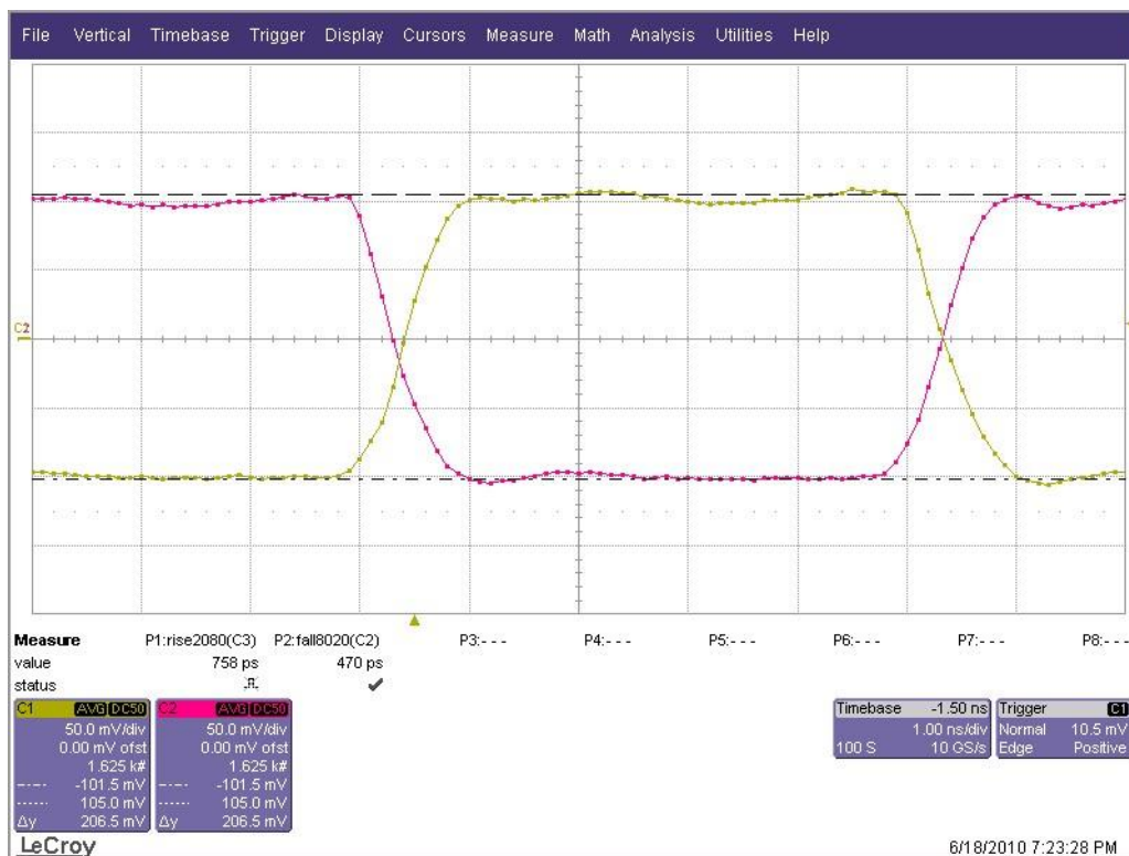
Figure 2.4. Typical Differential Output Waveform > 200 mV from Hardware Test
