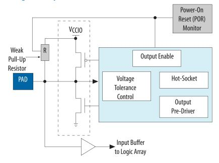
The POR circuit monitors the voltage level of power supplies and keeps the I/O pins tri-stated during power up. The weak pull-up resistor in Intel MAX 10 device I/O elements (IOE) keeps the I/O pins from floating. The voltage tolerance control circuit protects the I/O pins from being driven before  $V_{CCIO}$  and  $V_{CC}$  supplies are powered up. This prevents the I/O pins from driving out when the device is not in user mode.
