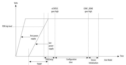
Note: Each individual power supply must reach the recommended operating range within the
