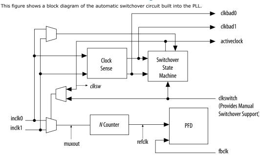
When the current reference clock is not present, the clock sense block automatically switches to the backup clock for PLL reference. You can select a clock source at the backup clock by connecting it to the inclk1 port of the PLL in your design.
