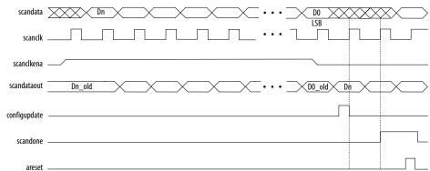
When reconfiguring the counter clock frequency, you cannot reconfigure the corresponding counter phase shift settings using the same interface. You can reconfigure phase shifts in real time using the dynamic phase shift reconfiguration
