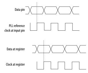
Source synchronous mode compensates for clock network delay, including any difference in delay between the following two paths:
