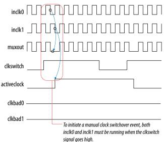
The clkswitch signal and automatic switch work only if the clock being switched to is available. If the clock is not available, the state machine waits until the clock is available.
