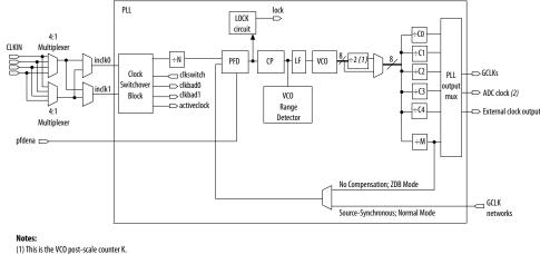
(1) This is the VCO post-scale counter K.(2) Only counter CO of PLL1 and PLL3 can drive the ADC clock.
