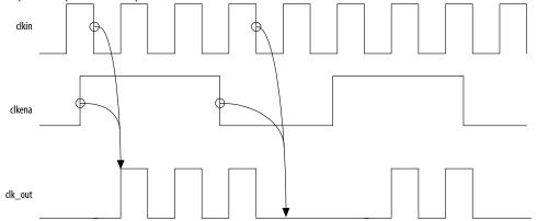
The clkena signal can also disable clock outputs if the system is not tolerant to frequency overshoot during PLL resynchronization.
