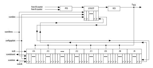
The counter settings are updated synchronously to the clock frequency of the individual counters. Therefore, not all counters update simultaneously.
