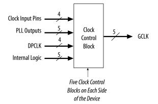
Out of these five inputs to any clock control block, the two clock input pins and two PLL outputs are dynamically selected to feed a GCLK. The clock control block supports static selection of the signal from internal logic.
