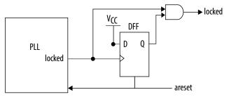
*Note:* If you use the Signal Tap II tool to probe the locked signal before the D flip-flop, the locked signal goes low only when areset is deasserted. If the areset signal is not enabled, the extra logic is not implemented in the ALTPLL IP core.
