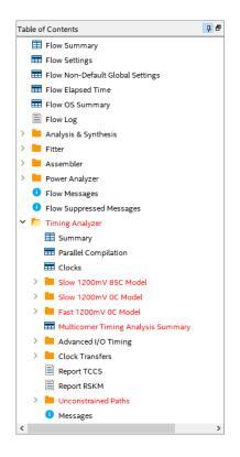
3.3.2.2 Expand **Slow 1200mV 85C Model** folder and click on **Setup Summary**. Here you can see the slack of clock-controlled signal.
