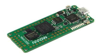
Software and hardware requirements to complete all exercises Software Requirements: Quartus<sup>®</sup> Prime Lite or Standard Edition version 18.0 or 18.1 Hardware Requirements: ARROW MAX1000 Board
