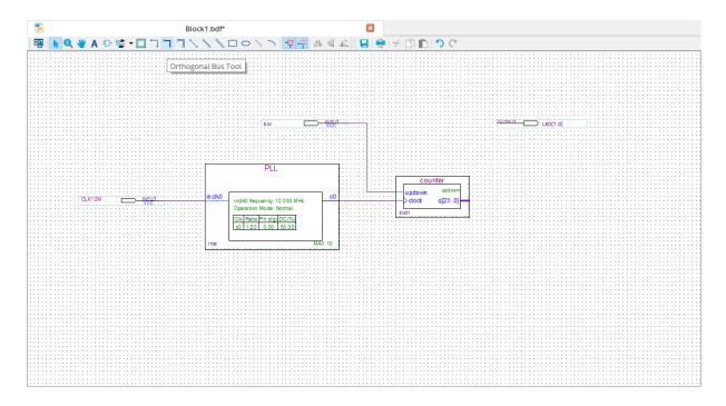
4.2.3.15 Using the bus tool create a connection coming out of the counter and one connection for the LEDs.
