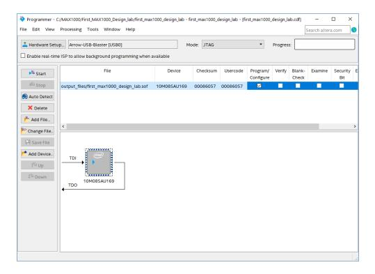
4.3.4.12 Click **Start** to program the board. When the configuration is complete, the Progress bar should show 100% (Successful).
