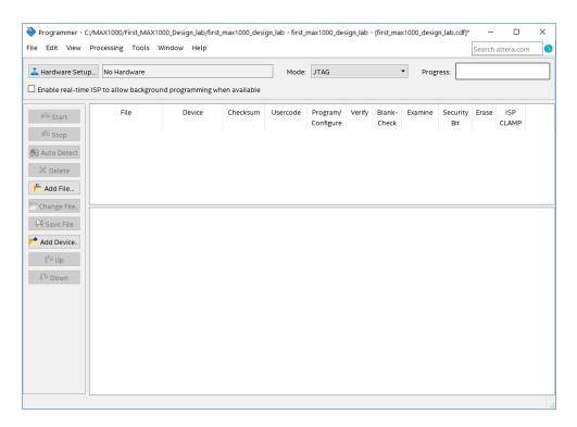
4.3.4.3 Click **Hardware Setup...** and double click **Arrow-USB-Blaster** entry in the Hardware Setup tab. The Currently selected hardware should now show Arrow-USB-Blaster [USB0] (depending on your PC, the USB port number may variant).
