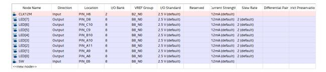
4.3.2.4 Double click in the I/O Standard column for any ten pins to open a drop-down list and change the 2.5V (default) to the specific I/O standard.
