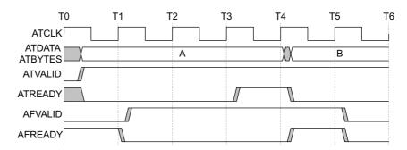
Figure 4-3 Flushing from a master that lacks internal storage
