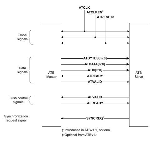
Figure 3-1 ATB signaling between master and slave
