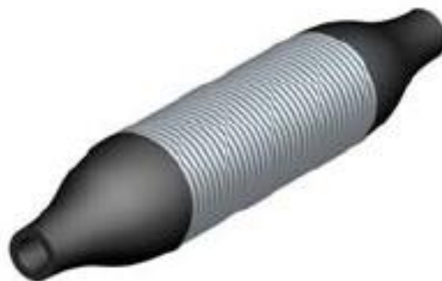
(b) Compressed spring
