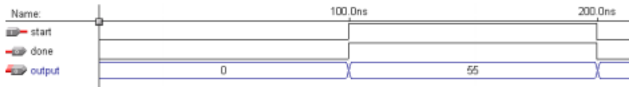
Figure 11.32. Behavioral model of the microprocessor for the summation algorithm.
