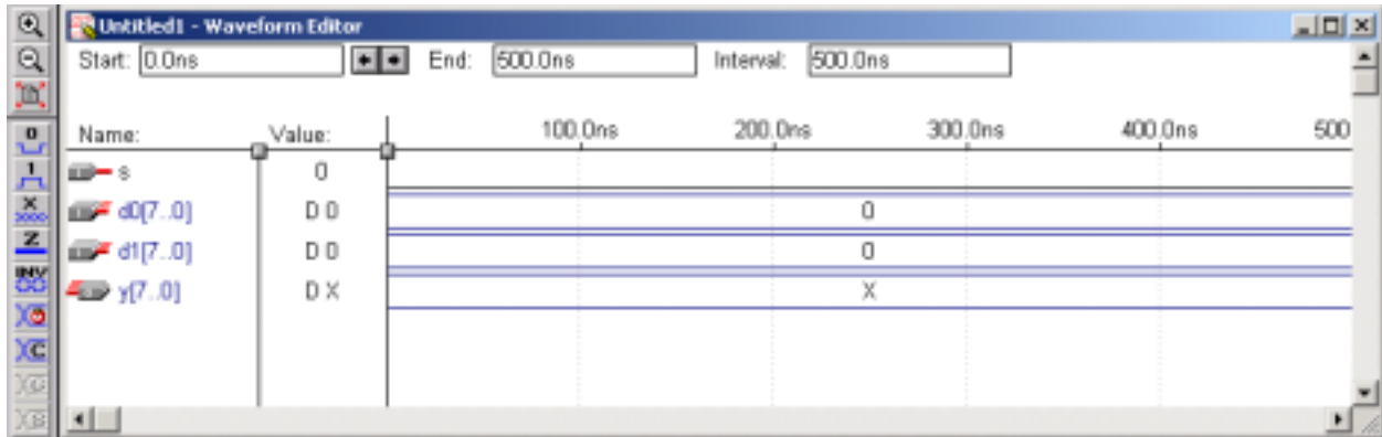
Figure A.12 Waveform Editor window after changing the value radix and fitting the entire time range inside the window. Notice also the toolbar buttons on the left.
