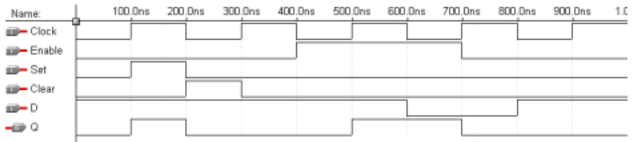
Figure 6.27 Simulation trace for the positive-edge-triggered D flip-flop with active-high enable and asynchronous set and clear inputs.
