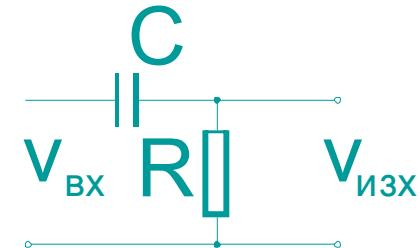
$$RC \frac{dv_{izx}}{dt} + v_{izx} = RC \frac{dv_{ex}}{dt}$$
