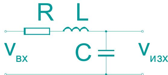
$$LC \frac{d^2 v_{izx}}{dt^2} + RC \frac{dv_{izx}}{dt} + v_{izx} = v_{ex}$$
