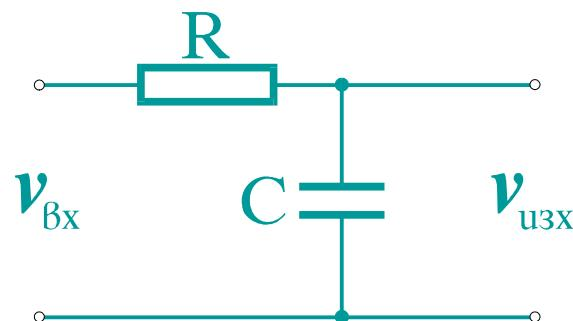
$$RC \frac{dv_{uzx}}{dt} + v_{uzx} = v_{bx}$$
