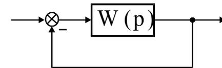
$$\begin{aligned} W_{y,v}(p) &= \frac{W(p)}{1+W(p)} = \\ &= \frac{10(2p+1)}{p(10p+1)} = \\ &= \frac{10(2p+1)}{1 + \frac{10(2p+1)}{p(10p+1)}} = \\ &= \frac{20p+1}{10p^2 + 21p + 10} \end{aligned}$$
