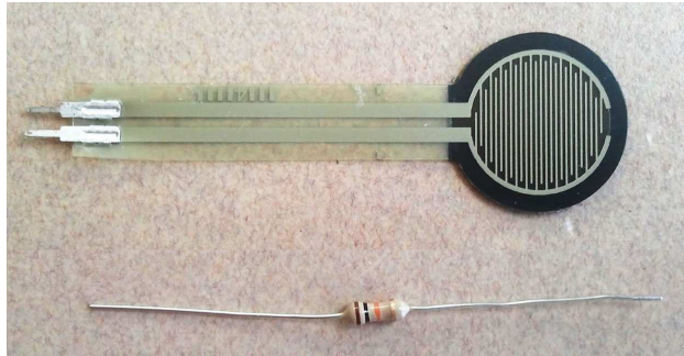
Figure 18—Package Delivery Detector resistors
