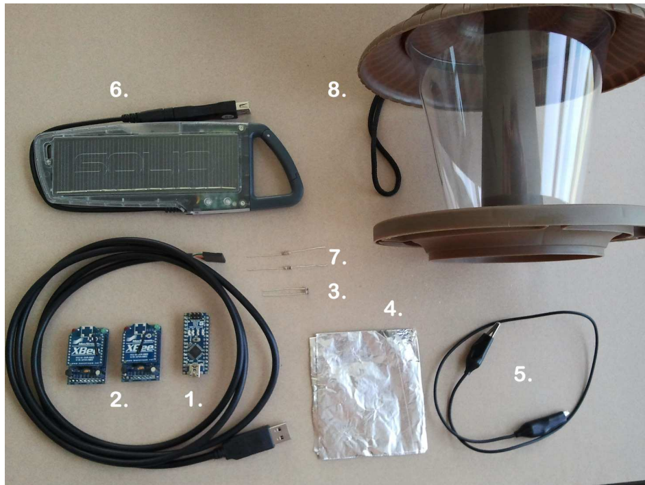
Figure 10—Tweeting Bird Feeder parts
