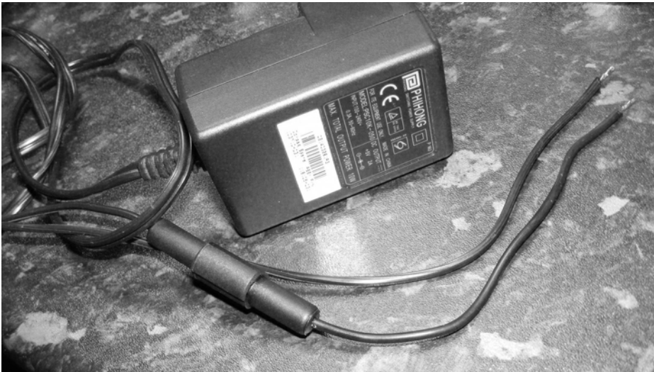
Figure 2-5. A repurposed 5 volt supply
