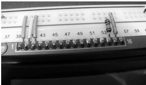
Figure 10-3. WordDune: LCD display at column 40 with ties and R2 installed
