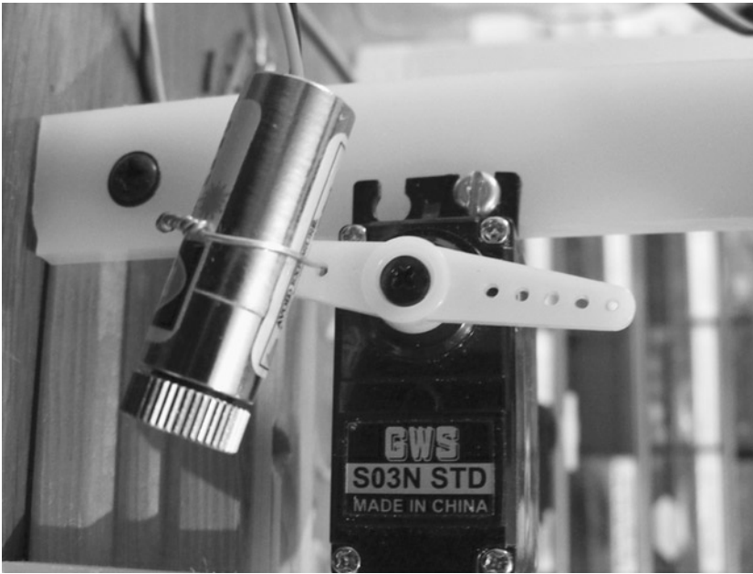
Figure 9-4. Laser diode mounted on servo motor
