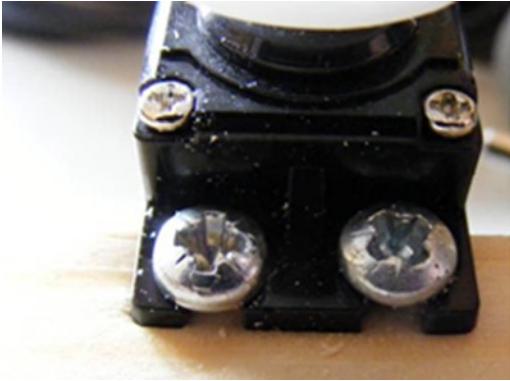
Figure 4-6. Using self-tapping cheesehead screws
