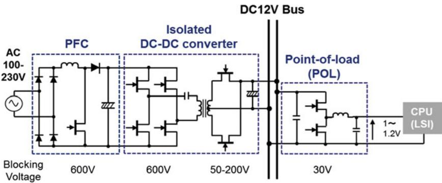
Fig. 11.18 Circuit diagram of a typical power supply system
