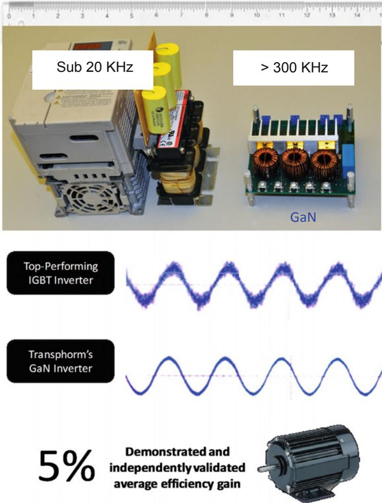
**Fig. 4.24** Motor drive with a sinusoidal signal. At the left is the filter required to condition the sub 20 kHz PWM signal employed in a Si drive versus the compact filter required to condition the 300 kHz signal used for a GaN-based motor drive. An increase in the efficiency of the motor results because of the lack of charging/discharging losses caused by the pulses in an unfiltered conventional IGBT inverter
