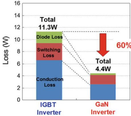
Fig. 11.17 Details of operating losses of inverter systems using GITs and IGBTs at the output power of 500 W
