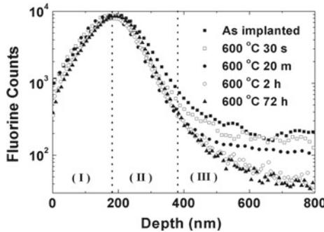
**Fig. 12.8** Depth profiles of fluorine after post-implantation annealing at 600 °C. This experiment was conducted on a sample implanted by 180 keV F ions with a dose of  $1 \times 10^{15}/\text{cm}^2$ , so that the peak F concentration is deep inside the bulk
