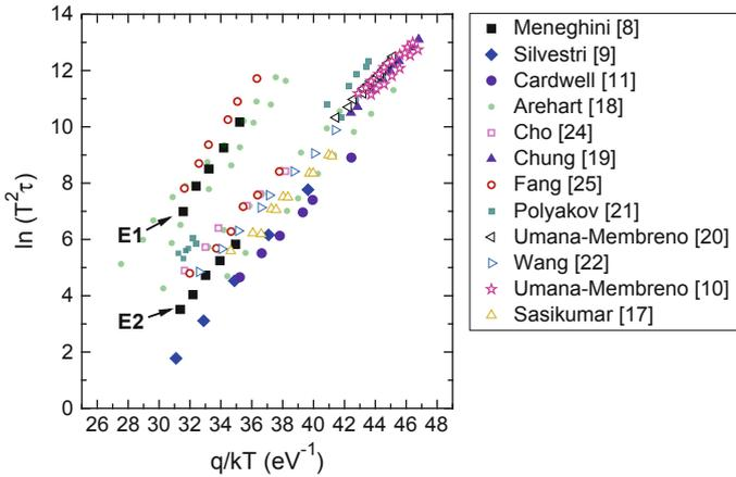
**Fig. 9.7** Arrhenius plot of the deep levels E1 and E2 detected by Meneghini et al. [62]. Activation energy of 0.82 and 0.63 eV is extrapolated, respectively. Comparison of the deep levels detected in Meneghini et al. [62] with previous works reported in the literature concerning devices with and without intentionally iron doping
