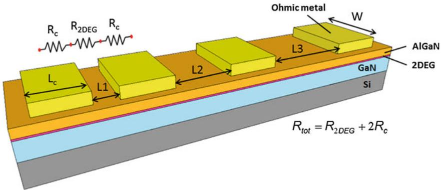
**Fig. 14.1** Schematic of the TLM structure on AlGaN/GaN with various contact spacings ( $L_1$ ,  $L_2$ ,  $L_3$ , ...). Resistances and other dimensions are as defined in the text
