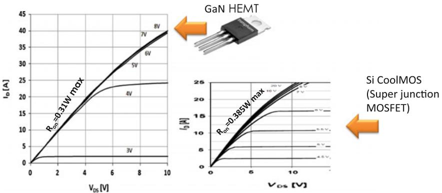
**Fig. 4.20** Cascode device IV curves compared with Si CoolMOS
