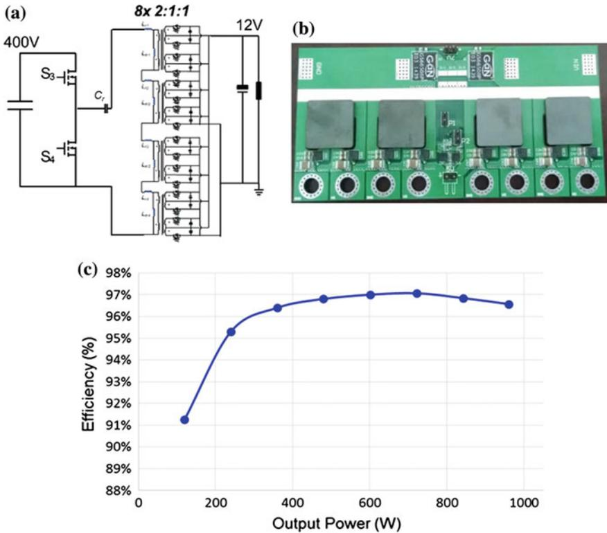
**Fig. 15.30** A further improved design of 1 kW LLC with matrix transformer: **a** circuit diagram, **b** prototype, and **c** measured efficiency
