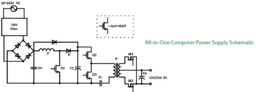
Fig. 10.9 GaN HEMT application in an AC-DC power supply with resonant DC-DC switching stage
