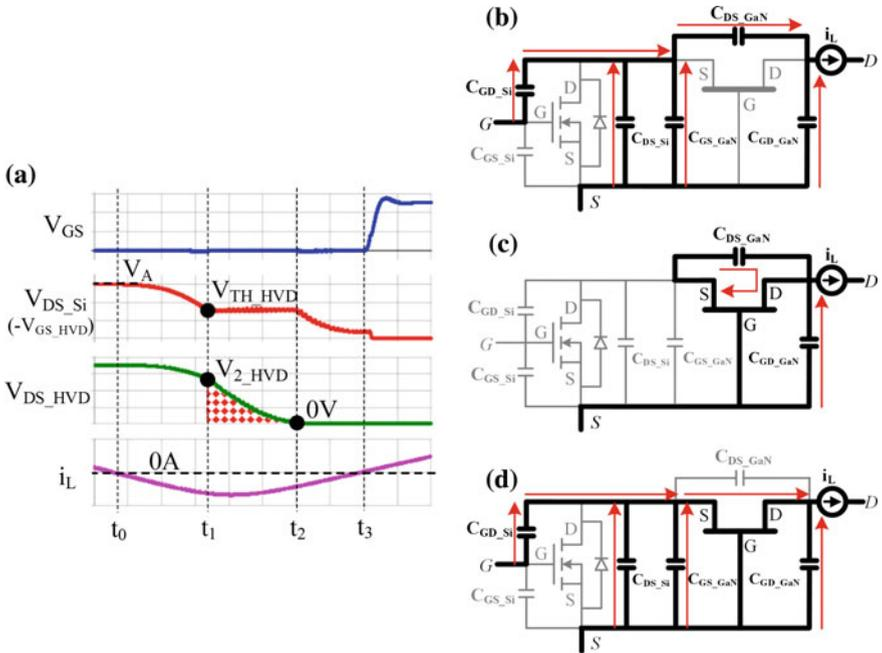
**Fig. 15.12** Voltage distribution of cascode GaN during ZVS turn-on transition: **a** GaN internal turn-on, **b** stage I:  $t_0-t_1$ , **c** stage II:  $t_1-t_2$ , and **d** stage III:  $t_2-t_3$
