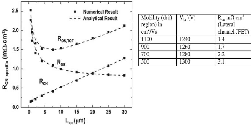
**Fig. 5.9**  $R_{on}$  of CAVET is comprised of the channel and the drift region resistance. The plot captures both of those components as a function of  $L_{ap}$ . Total  $R_{on}$  as a function of the electron mobility in the drift region is listed. Bulk GaN mobility will play a key role in distinguishing GaN vertical devices from SiC counterparts
