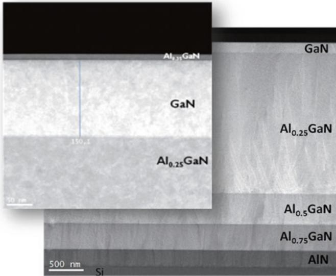
**Fig. 3.1** TEM image of the full GaN-on-Si epitaxial stack. The *upper part*, i.e., active region of the stack is magnified in the *inset*
