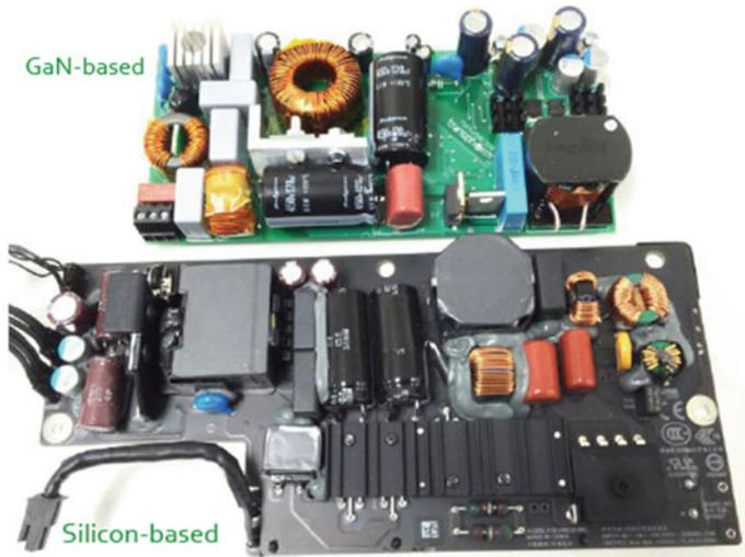
**Fig. 10.10** GaN-based 250-W power supply showing significant size reduction versus a Si MOSFET-based version. The cascode GaN allows use of industry-standard drivers and controllers
