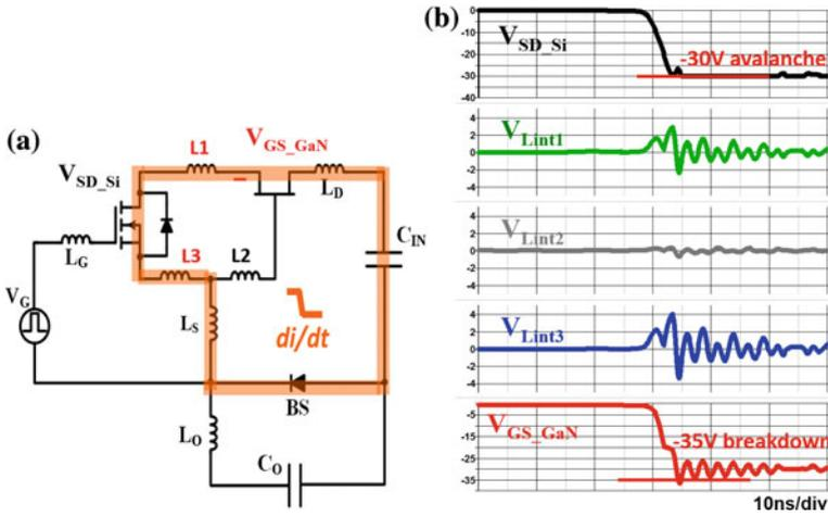
**Fig. 15.9** Gate breakdown mechanism: **a**  $di/dt$  loop on circuit and **b** simulation waveforms
