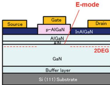
Fig. 11.21 Schematic cross section of the fabricated p-gate GIT employing InAlGaN/GaN heterostructure with high sheet carrier concentration
