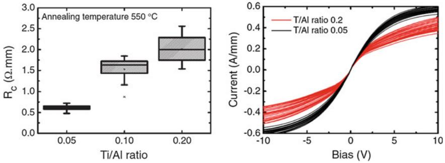
**Fig. 3.13** Contact resistance, *left*, versus Ti/Al ratio, *right*, maximum TLM current for metal stacks with two different Ti/Al ratios
