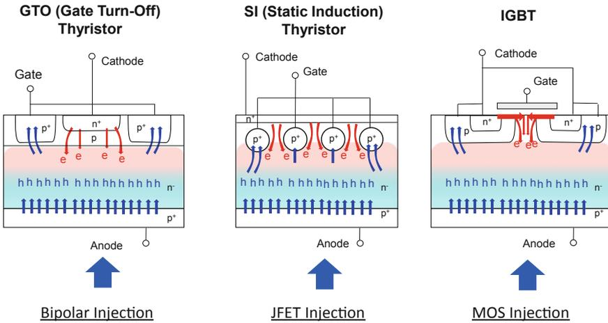
**Fig. 1.21** Representative Si power devices that use conductivity modulation in the drift region. You can see the difference of electron leading structure into the drift region to occur the hole injection from the bottom p region
