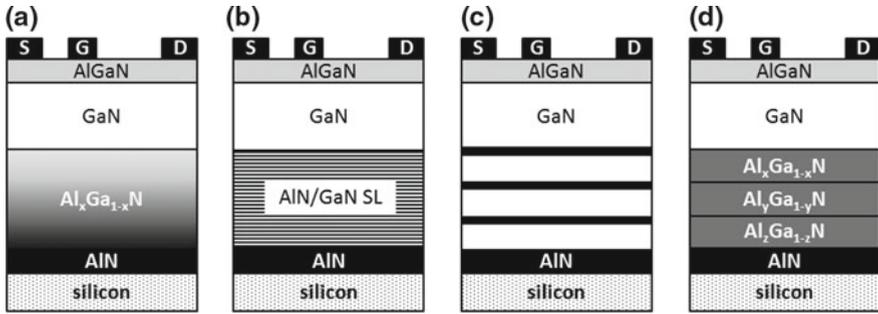
**Fig. 2.5** Schematics of transistors with different base layers for strain management on Si substrates: **a** graded AlGaIn layer, **b** AlN/GaN superlattice (SL), **c** AlN interlayers, and **d** step-graded  $\text{Al}_x\text{Ga}_{1-x}\text{N}$  layers where  $x < y < z$
