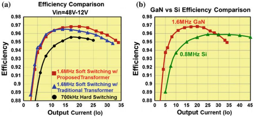
Fig. 15.28 Efficiency curves showing **a** hard-switching/soft-switching comparison and **b** GaN transistors versus Si MOSFETs
