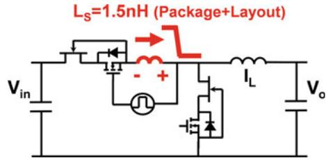
**Fig. 15.17** High  $di/dt$  induces voltage spike across CSI
