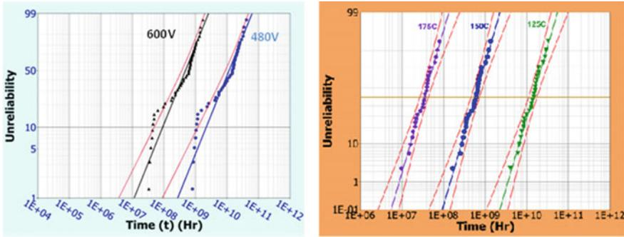
**Fig. 10.13** High-voltage off-state (*left*)—and high-temperature on-state (*right*)—accelerated testing at multiple voltages (HVOS) and multiple temperatures (HTOS) to determine intrinsic lifetimes under these wear-out mechanisms
