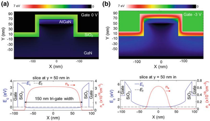
**Fig. 6.7** Simulated 2D plots of the conduction band edge of the 70-nm-side-wall depletion-mode tri-gate AlGaN/GaN MISFET at gate bias of 0 (a) and  $-3$  V (b) with 1D slices at  $Y = 50$  nm positions. Adapted from [38]
