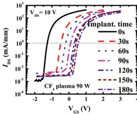
**Fig. 12.2** Transfer characteristics of AlGaN/GaN HEMTs with different fluorine plasma ion implantation times
