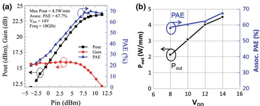
**Fig. 4.15** 10 GHz load pull of N-polar deep recess device with a designed gate length of 150 nm and 47 nm GaN cap passivation in access regions. **a** Power sweep at 14 V bias and **b** maximum power and associated PAE versus drain bias voltage show excellent scaling in power density and PAE versus drain bias [61]. Measurement provided by Maury Microwave
