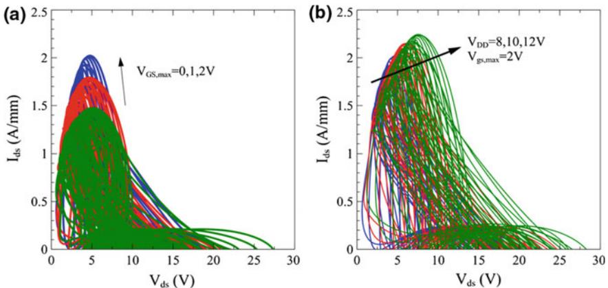
**Fig. 4.13** Families of dynamic loadlines measured over multiple load impedances in active harmonic vector load pull at 6 GHz, plotted for **a**  $V_{DD} = 8$  V bias with  $P_{IN}$  corresponding to a maximum  $V_{GS}$  of 0, 1, or 2 V during the RF cycle, and **b**  $V_{DD} = 8, 10,$  and 12 V bias at  $P_{IN}$  corresponding to a peak  $V_{GS}$  of 2 V during the RF cycle [61]. The high RF current capability of N-polar deep recess devices. Measurement provided by Maury Microwave
