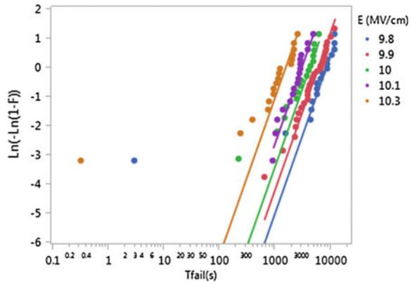
**Fig. 14.22** Normalization of the TDDB data of Fig. 14.21 to one stress field, using the P-F field acceleration model. Weibull slope  $\beta = 2.35$
