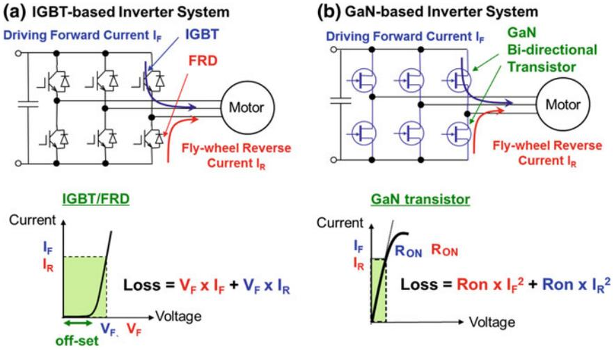
**Fig. 11.13** Operations of **a** a conventional IGBT inverter system and **b** GaN-based one with the description of forward and reverse conduction losses
