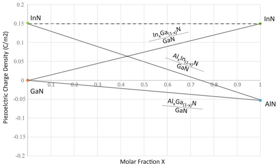
**Fig. 1.6** Theoretically calculated piezoelectric polarization charge density for three ternary alloys, namely  $Al_xGa_{(1-x)}N$ ,  $In_xGa_{(1-x)}N$ , and  $Al_xIn_{(1-x)}N$  over GaN substrate, as a function of the mole fraction  $x$ . The calculation is based on Ambacher et al. [9]
