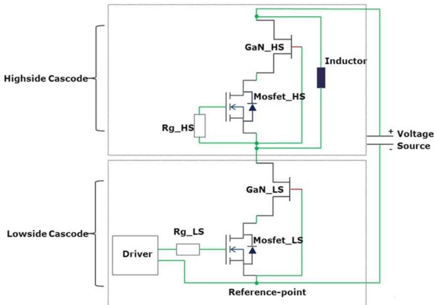
Fig. 8.20 Schematic of the half-bridge GaN cascode board
