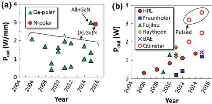
**Fig. 4.7** Yearly progression in reported W-band (75–110 GHz) GaN power performance, including both MMIC and single device results [34, 36, 37, 39, 104–115]: **a** maximum GaN output power density for Ga-polar versus N-polar material. Material technology is labeled, (Al, Ga)N referring to both AlGaN/GaN and AlN/GaN devices. **b** Maximum single-chip output power levels, some measurements (labeled) were pulsed at a low duty cycle to reduce self-heating effects giving increased the output power
