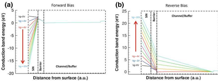
**Fig. 14.13** Band conduction ( $E_c$ ) band diagram under **a** forward bias condition; **b** reverse bias condition
