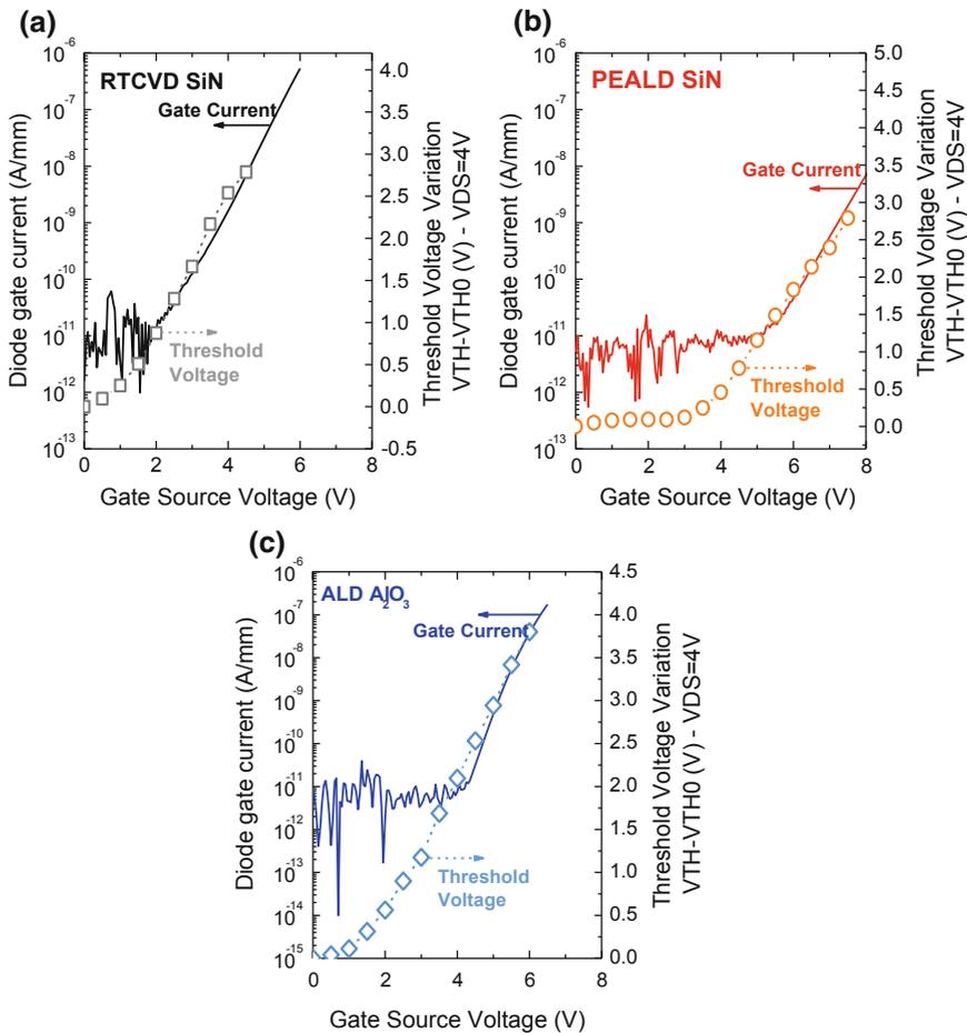
**Fig. 9.20** Correlation between the threshold voltage dynamic shift (*void circles*) and the gate leakage forward current (*solid line*) for different dielectric materials ( $SiN$ ,  $Al_2O_3$ ) and deposition techniques (plasma-enhanced atomic layer deposition and rapid thermal chemical vapor deposition)
