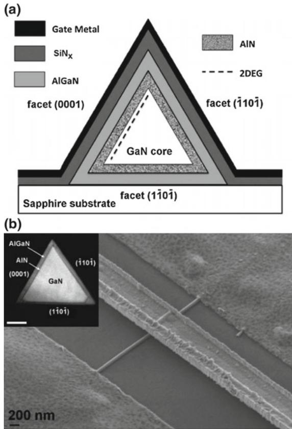
as shown in Fig. 6.2. Devices presented intrinsic current-gain cutoff frequency ( $F_T$ ) of 5 GHz as well as an intrinsic maximum available gain ( $F_{MAX}$ ) cutoff frequency of 12 GHz. These results show the potential of GaN-based nanowire FETs also for microwave applications.
