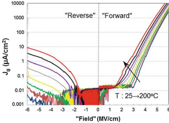
**Fig. 14.12**  $J_g$ - $E_g$  curves measured on the gate capacitor structures as a function of ambient temperature
