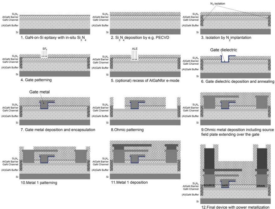
Fig. 3.3 Schematic illustration of the main process steps to obtain GaN-based power transistors
