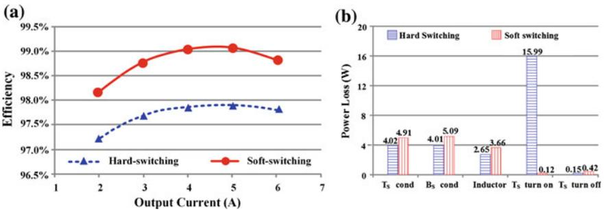
**Fig. 15.8** Soft switching versus hard switching **a** efficiency comparison and **b** loss breakdown at 6 A
