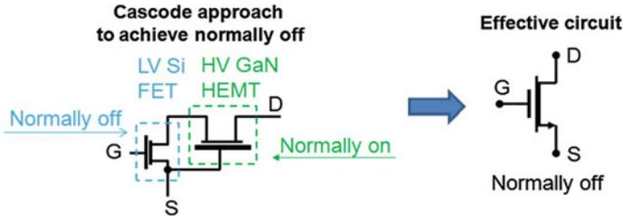
Fig. 10.1 Schematic of the cascode high-voltage GaN HEMT
