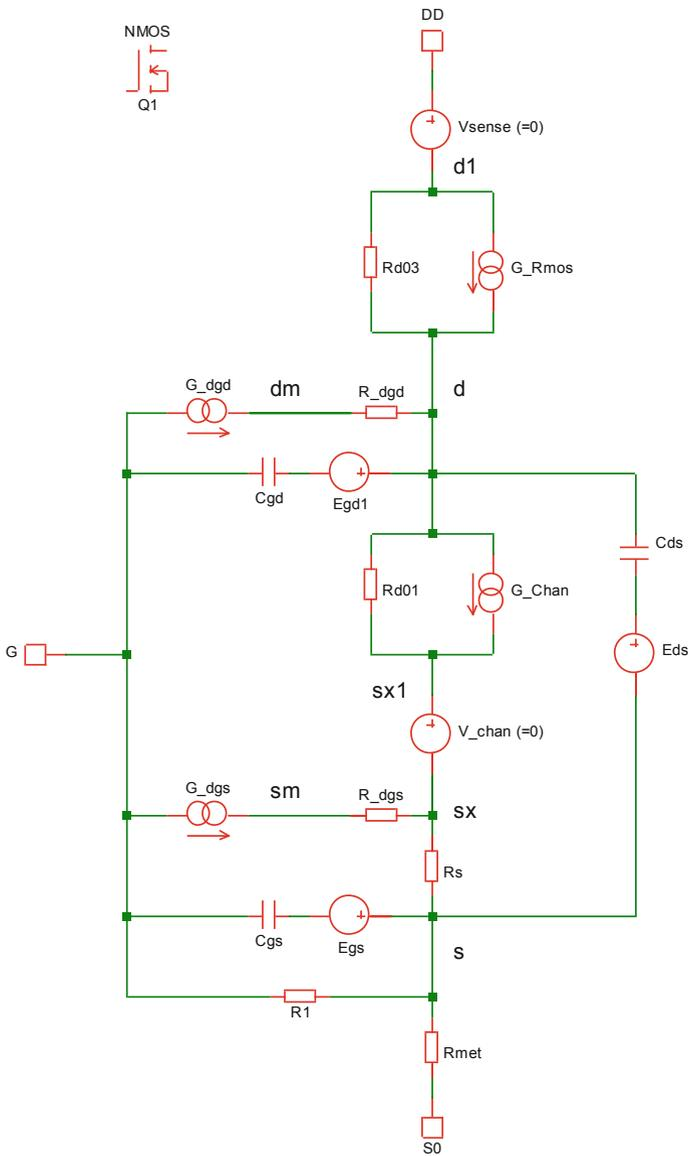
**Fig. 8.12** Example of a GaN Spice model for a normally-off pGaN concept
