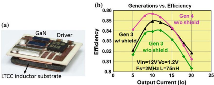
**Fig. 15.24** 3D integrated POL converters with EPC GaN devices: **a** prototype of 3D integrated POL converter and **b** test results of converter efficiency
