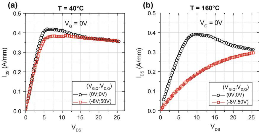
**Fig. 9.14** Pulsed  $I_{D-S}$ - $V_{D-S}$  characteristics of an AlGaIn/GaN/AlGaIn MIS-HEMT acquired at **a** 40 °C and **b** 160 °C. When exposed to the off-state quiescent bias point, the devices under test experience an increase of the dynamic  $R_{ON}$ . This effect is positive temperature-dependent, thus of great concern for high-temperature operations. Data from Bisi et al. [98]
