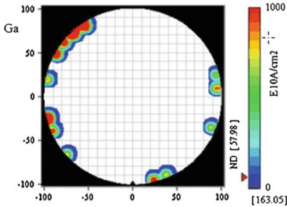
**Fig. 3.16** TXRF analysis of a Si wafer surface after contact with the chuck of the MOCVD epi tool
