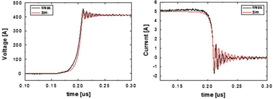
**Fig. 8.25** Simulated and measured turn-on transition of a normally-on GaN device at 400 V off-state voltage and for a load current of 5 A
