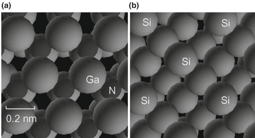
**Fig. 12.3** Top view of **a** Ga-faced (0001) GaN wurtzite crystal, and **b** (100) Si crystal. The same physical scale is used in **(a)** and **(b)**. Even Si features larger lattice constant (5.43 Å), there is little opening along the incident direction
