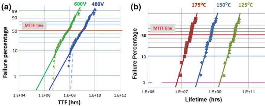
**Fig. 4.19** Transphorm 600 V GaN accelerated lifetime test results: **a** voltage accelerated reliability characterization. Data collected over 900–1200 V and plotted at 600 and 480 V, using inverse power law model. MTTF  $8 \times 10^7$  h at 600 V. **b** Temperature accelerated reliability characterization. Data collected at  $T_j$  from 318 to 362 °C which showed an activation energy of 1.84 eV and no indication of early failure modes. MTTF of  $3 \times 10^7$  h at 175 °C
