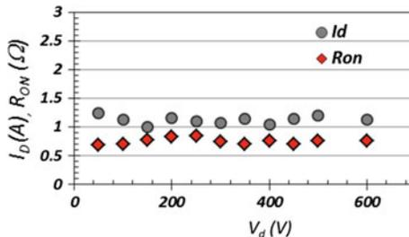
**Fig. 4.16** Dynamic current and on-resistance measured directly in a DC–DC converter, showing low dispersion over the full 600 V operating range. Figure courtesy of Transphorm
