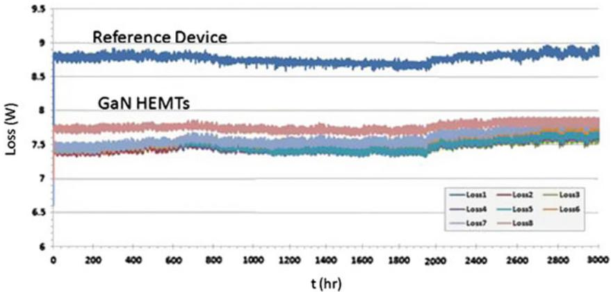
**Fig. 10.12** Loss plot for GaN HEMTs along with a reference device all operating under 300 kHz, 175 °C, 400 W, 1:2 boost switching conditions for the HTOL test. No change observed in performance and key parameters (before/after) following 3000 h of operation
