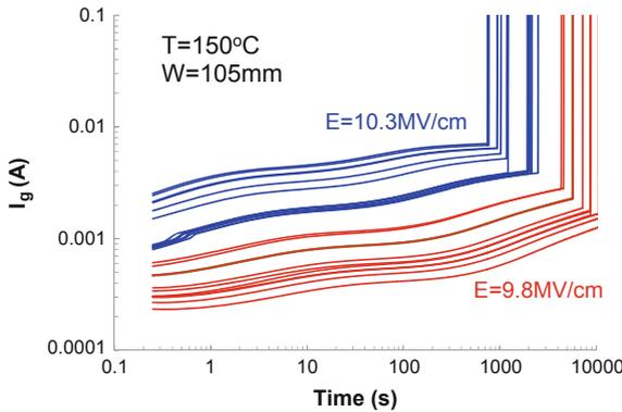
**Fig. 14.20**  $I_g$ -time curve characteristics measured on  $W = 105$  power transistors. Constant forward gate field stress (TDDB),  $T = 150^\circ\text{C}$
