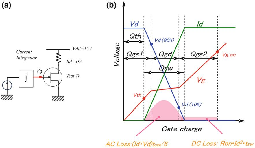
Fig. 1.17 The typical measurement system of  $R_{on}$   $Q_g$  and observed current/voltage waveform during the switching, where  $Q_g$  represents the sum of  $Q_{gs1}$ ,  $Q_{sw}$ , and  $Q_{gs2}$
