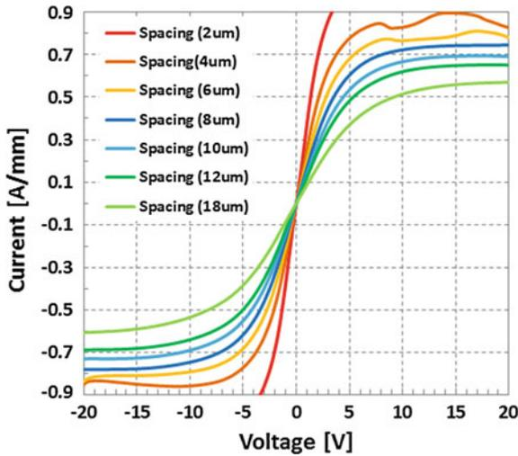
Fig. 14.2 Electrical characteristics of the TLM structures measured at room temperature for different spacing ranging from 2 to 18  $\mu\text{m}$
