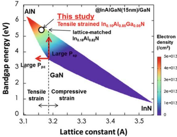
Fig. 11.20 Bandgap energies of InAlGaN quaternary alloy system plotted as a function of the lattice constants
