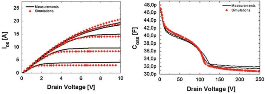
**Fig. 8.9** Experimental (*solid*) and simulated (*symbols*) IV curves and CV curves for a normally-on GaN HEMT
