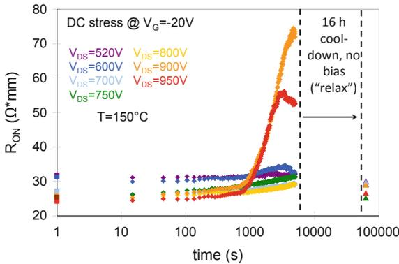
**Fig. 14.26**  $R_{on}$  as a function of stress time for different  $V_{ds\_stress}$  conditions from 520 V up to 950 V and  $T = 150\text{ }^{\circ}\text{C}$ . Stress is stopped after 6000 s, after which the devices are cooled down (“relax”). Devices fully recover after 16 h of relax. Note the dynamics in the static  $R_{on}$  at  $V_{ds} = 900$  and 950 V, showing a partial recovery even during the off-state stress
