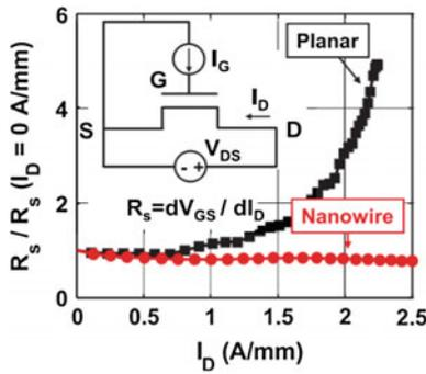
**Fig. 6.12** Source resistance over a range of drain current density for a nanowire channel device and a planar device. Adapted from [50]
