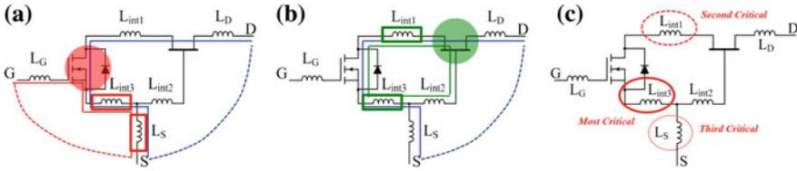
**Fig. 15.3** Common-source inductance distribution in cascode GaN device: **a** in a Si device, **b** in a GaN device, and **c** for cascode structure
