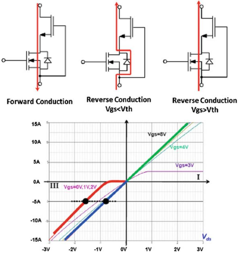
**Fig. 10.5** Current paths in the cascode GaN switch for three operating modes, and the corresponding I-V characteristic
