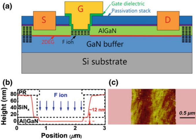
**Fig. 12.15** **a** Cross section of a fabricated E-mode MIS-HEMT. **b** Side wall profile of the gate region after F-implantation (solid line in red) and the outline of gate region before F-implantation. **c** Surface morphology of the recessed gate region
