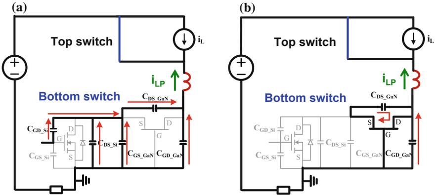
Fig. 15.14 Equivalent circuits **a**  $t_0-t_1$  equivalent circuit and **b**  $t_1-t_2$  equivalent circuit
