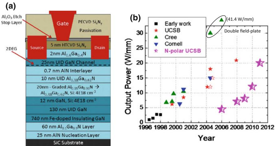
**Fig. 4.9** **a** Cross-section (not to scale) of N-polar MISHEMT which demonstrated 20.7 W/mm output power density (figure by Kolluri [69]). **b** Maximum RF output power density by year for Ga-polar and N-polar GaN devices (figure after S. Keller)
