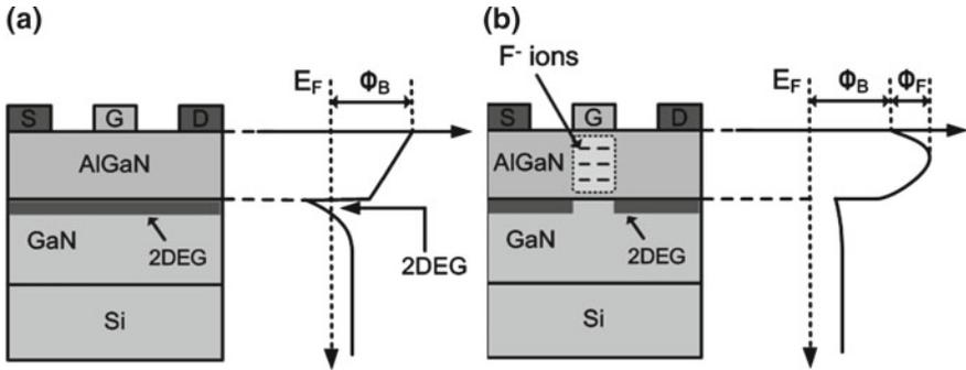
**Fig. 12.1** Cross section and the conduction band profiles of standard **a** normally on and **b** normally off AlGaN/GaN HEMTs. The normally off HEMT features F<sup>-</sup> ions incorporated in the AlGaN barrier by plasma ion implantation
