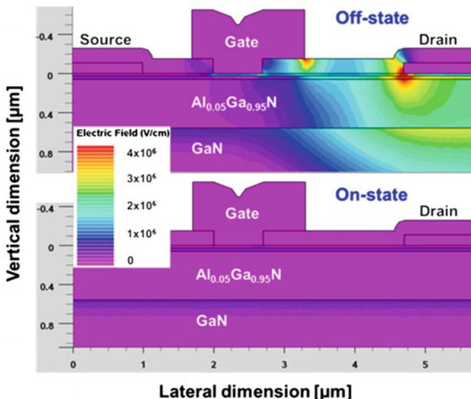
**Fig. 13.4** Visualization of internal electric field distribution after switching a GaN power transistor from off-state to on-state condition (see also [2, 16]): Off-state condition: simulation of electric field distribution of a GaN HFET at reverse bias condition and at a drain voltage of 300 V. The 2DEG is fully depleted. On-state condition: Simulation of electric field distribution at steady-state on-state condition (drain voltage 0 V). The 2DEG is fully conductive in this case
