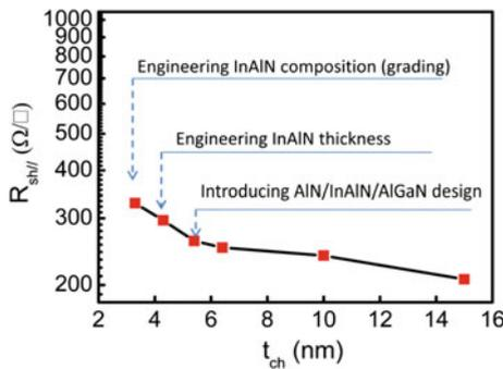
**Fig. 4.11** Trend of sheet resistance vs. channel thickness for InAlN-based backbarrier HEMTs, and design features used to reduce sheet resistance for thinner channels, culminating in 329  $\Omega$  sheet resistance for a 3.3 nm channel [87]. Figure by Lu [119]
