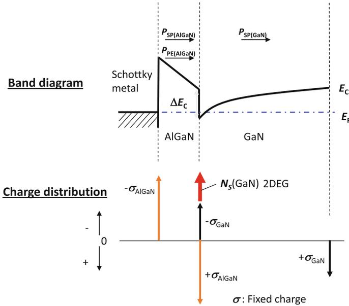
**Fig. 1.8** Band diagram of Schottky junction formed over  $\text{Al}_{0.25}\text{Ga}_{0.75}\text{N}$  grown on Ga-face GaN
