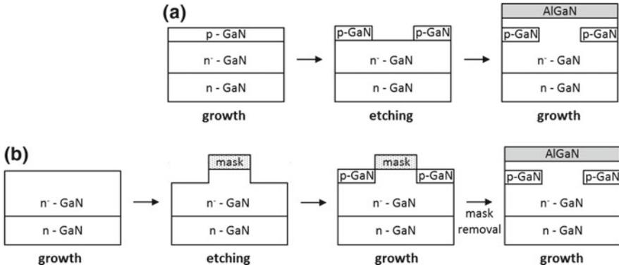
**Fig. 2.12** Process flow for the fabrication of a vertical FET (CAVET) via regrowth of **a** aperture and top HEMT and **b** p-GaN current-blocking region and top HEMT
