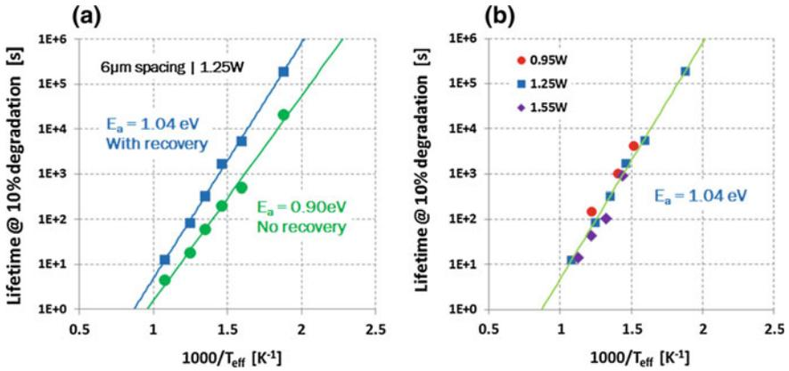
**Fig. 14.9** **a** Arrhenius plot: mean time-to-failure versus the inverse of the effective temperature extracted for step stress with and without recovery step after stress at  $1.25\text{ W}$  on  $6\mu\text{m}$  contact spacing; **b** Arrhenius plot: mean time-to-failure versus the inverse of the junction temperature extracted for step stress with recovery step after stress  $0.95$ ,  $1.25$ , and  $1.55\text{ W}$  on  $6\mu\text{m}$  contact spacing
