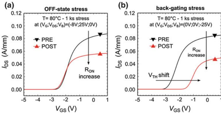
**Fig. 9.17**  $I_D$ – $V_G$  characteristics ( $V_{DS} = 1 V$ ) acquired prior to and after **a** off-state stress and **b** back-gating stress. When exposed to back-gating stress, the device experiences not only the dynamic  $R_{ON}$  increase, but also a positive  $V_{TH}$  shift of +1.43 V, proving that the buffer charge trapping happens also within the intrinsic device region, below the gate contact. Data from Bisi et al. [98]
