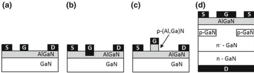
**Fig. 2.1** Schematics of different AlGaN/GaN transistors: **a** D-mode structure and E-mode structures with **b** recess gate or **c** p-(Al,Ga)N cap layer, **d** vertical transistor (CAVET). *S* source, *D* drain, *G* gate
