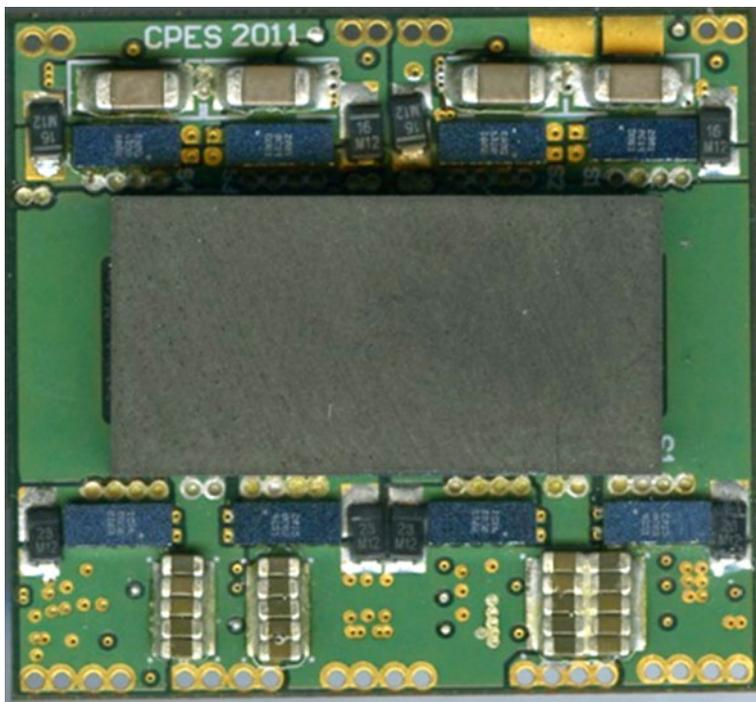
**Fig. 15.27** 48–12 V, 1.6 MHz isolated buck converter with GaN transistors
