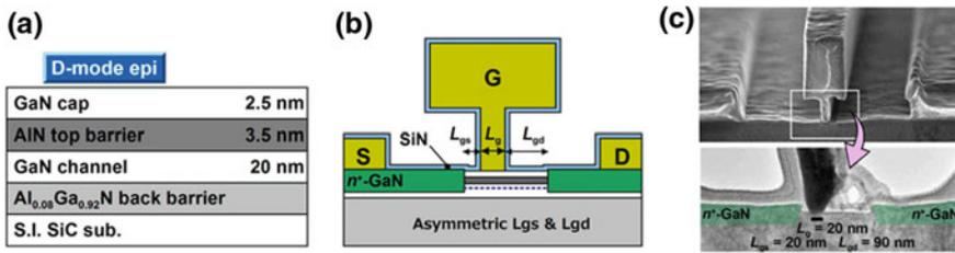
**Fig. 4.6** **a** Epitaxy design, **b** device schematic cross-section and **c** TEM image of HRL Gen-IV device with 20 nm gate length, capable of record GaN  $f_t$  and  $f_{max}$  [35]
