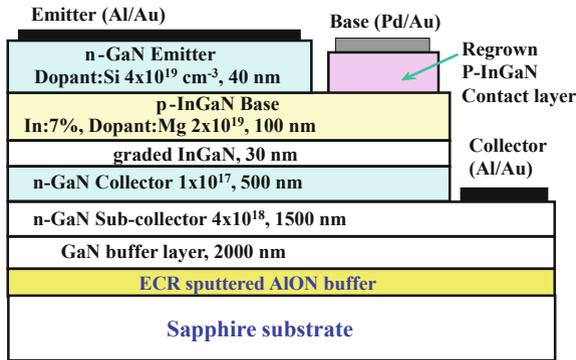
**Fig. 1.24** Experimentally fabricated GaN/InGaN DHBT structure with regrown P-InGaN base contact layer
