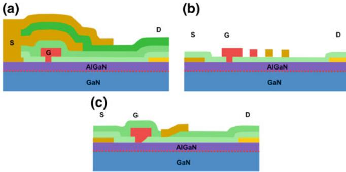
**Fig. 13.11** Different field plate approaches for breakdown voltage enhancement and for reducing dispersive effects (according to [16]): **a** stacks of source-connected field plates in conjunction with an asymmetric T-gate structure; **b** multiple grading field plates which can be deliberately biased at different potentials; and **c** slanted field plate structures
