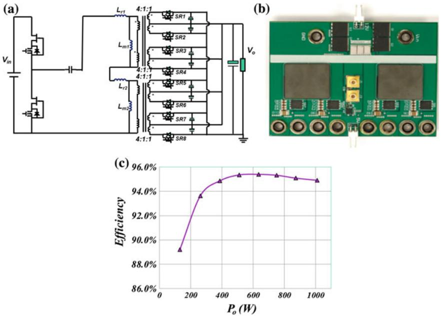
Fig. 15.29 Topology, prototype, and efficiency of 1 kW 400/12 V LLC resonant converter with matrix transformer: **a** circuit diagram, **b** prototype, and **c** measured efficiency
