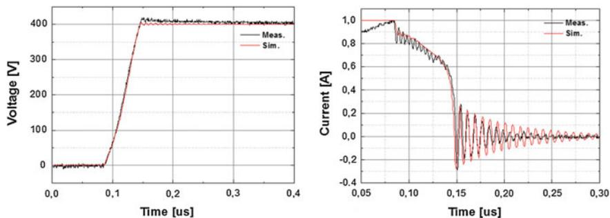
**Fig. 8.16** Simulated and measured turn-off transition of a pGaN device at 400 V off-state voltage and for a load current of 1 A
