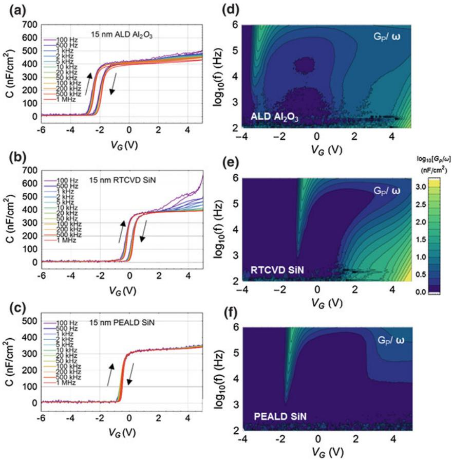
**Fig. 9.19** a–c C–V–f measurements and d–f normalized parallel conductance as a function of frequency and gate voltage for the three tested wafer. Reprinted with the permission from Ref. [131] © 2015 Elsevier Ltd
