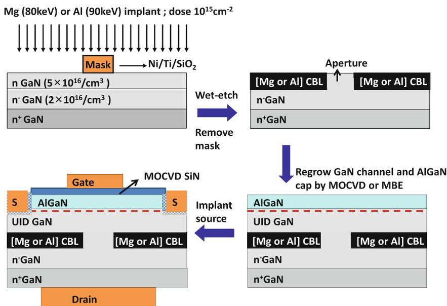
**Fig. 5.11** A schematic of a CAVET process flow. Here implanted CBL scheme has been adopted. Activation of the implanted species (not shown in the flow) occurs after the implantation stage. Regrowth can be accomplished by both MOCVD and MBE techniques. However, with Mg implantation, low-temperature regrowth is necessary to prevent Mg from out diffusing into the regrown layers
