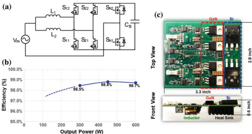
Fig. 15.31 GaN-based MHz totem-pole PFC **a** topology, **b** measured efficiency, and **c** prototype
