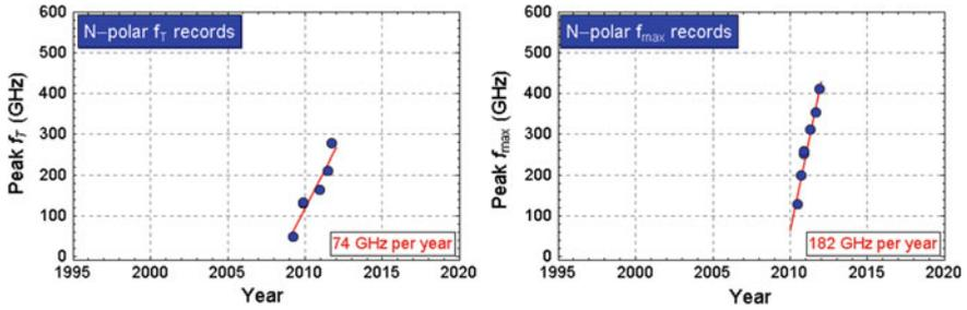
Fig. 4.12 Trend of record  $f_i$  and  $f_{max}$  versus year for N-polar HEMTs. Figure by Denninghoff [74]
