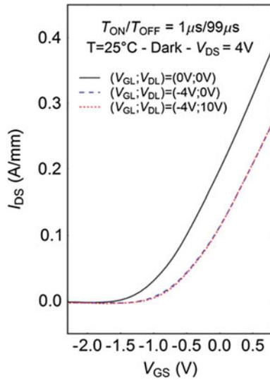
**Fig. 7.5** Pulsed  $I_{ds}-V_{gs}$  data for an AlGaIn/GaN HEMT with a Ni/Au gate and without surface passivation (Set C from text). Note that the response to the  $V_{gs} = -4$  V fill pulse depends strongly on  $V_{ds}$ , suggesting that the defects causing reduced  $I_{ds}$  are located in the access region and not under the gate. From Ref. [15]
