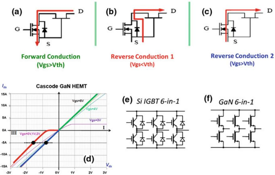
**Fig. 4.21** a–c The forward and reverse conduction modes of the Transform cascode and **d** their current versus voltage behavior, illustrating the bidirectional nature of these devices. A three phase inverter with **e** silicon IGBT devices and diodes, and **f** bidirectional GaN devices which do not require external high-voltage diodes
