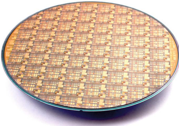
**Fig. 3.6** Photograph of a 200-mm processed GaN-on-Si wafer
