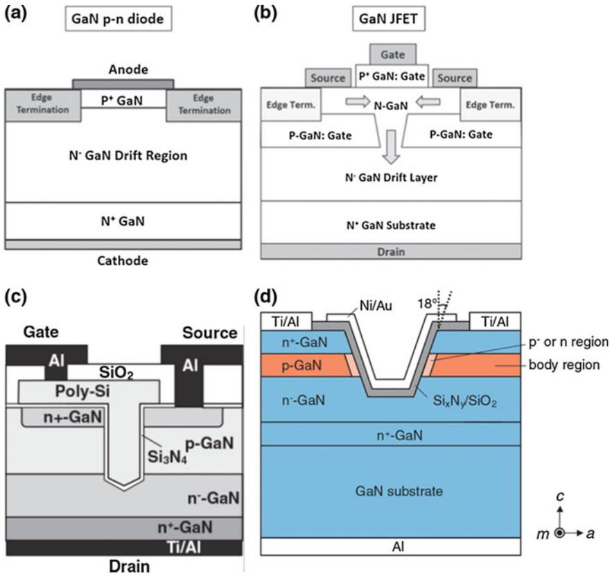
**Fig. 2.8** Schematics of vertical GaN devices: **a** p–n diode, **b** JFET, and **c** and **d** MISFETs. **a**, **b** Reproduced with permission from Ref. [132], Copyright 2015, IOP Publishing. All rights reserved. **c** Reprinted with permission from Ref. [4], Copyright 2014, the Japan Society of Applied Physics. **d** Reprinted with permission from Ref. [131], Copyright 2008, the Japan Society of Applied Physics
