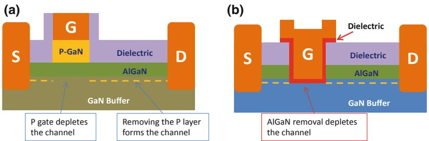
**Fig. 4.18** Methods for obtaining enhancement mode devices: **a** junction gated HEMTs (Panasonic, GaN systems). Disadvantage: low threshold voltages. **b** Channel etch-through MOSFET. Disadvantage: device and dielectric not qualified
