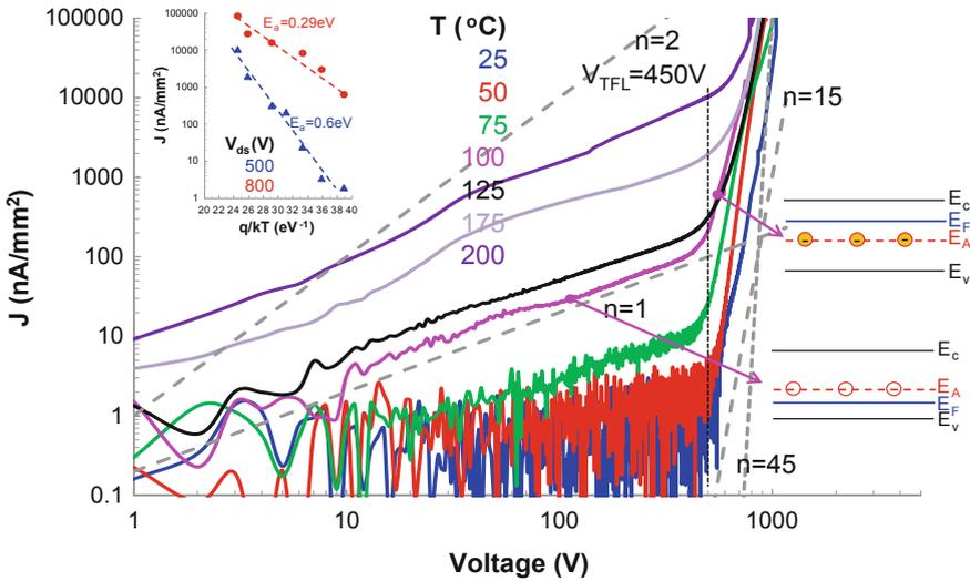
**Fig. 14.24**  $\ln(J)$ – $\ln(V)$  characteristic of the vertical leakage current as a function of temperature. The trap filling voltage  $V_{TFL}$  is the voltage at which all acceptor traps are ionized (see [28]), resulting in depinning of the Fermi level. Note the Ohmic conduction ( $n = 1$ ) till  $V = V_{TFL}$ . Above  $V_{TFL}$ , the current through the buffer increases rapidly. Electrons are injected from the Si substrate by thermionic emission with  $E_a = 0.6$  eV
