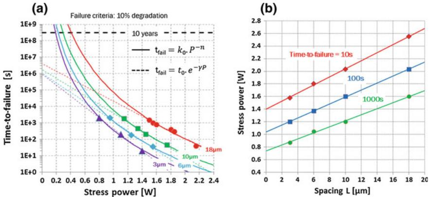
**Fig. 14.7** **a** Evolution of time-to-failure extracted at 10 % degradation as a function of constant stress power at 125 °C for different contact spacing. Data are fitted by means of power law (continuous line) and of exponential law (dashed line). **b** Stress power as a function of contact spacing for extrapolated time-to-failures 10, 100, and 1000 s
