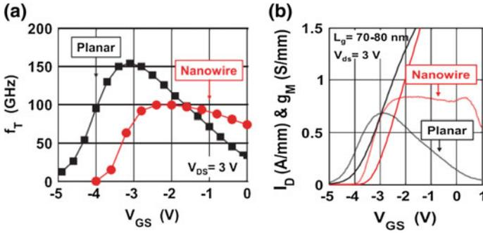
**Fig. 6.11** a Short-circuit current gain for a range of input voltages. b DC transfer characteristics of a nanowire channel device and a planar device [48]
