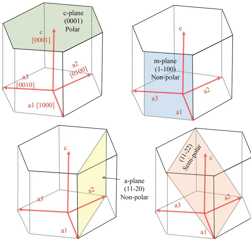
**Fig. 1.9** Representative crystal planes that have little polarization effect. Note that a-plane and m-plane are called nonpolar plane, while (0012) plane is called semi-polar plane
