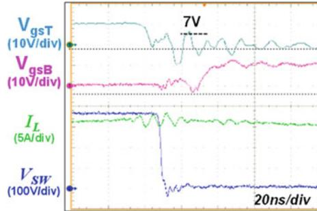
**Fig. 15.18** Smaller voltage spike with less CSI
