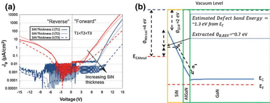
**Fig. 14.19** **a**  $J_g$ - $E$  curves measured on the gate capacitor as a function of temperature for three different SiN thicknesses. The blue-colored lines represent the data measured at 25 °C and the red-colored lines represent the data measured at 200 °C; **b** band diagram showing the estimated intrinsic defect energy within the SiN film (*Electron affinity for the MOCVD SiN film was assumed to be  $\sim 2 \text{ eV}$  for this calculation*)
