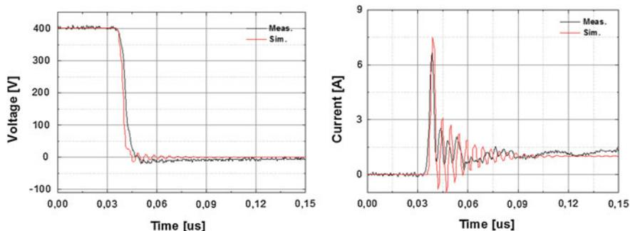
**Fig. 8.17** Simulated and measured turn-on transition of a pGaN device at 400 V off-state voltage and for a load current of 1 A
