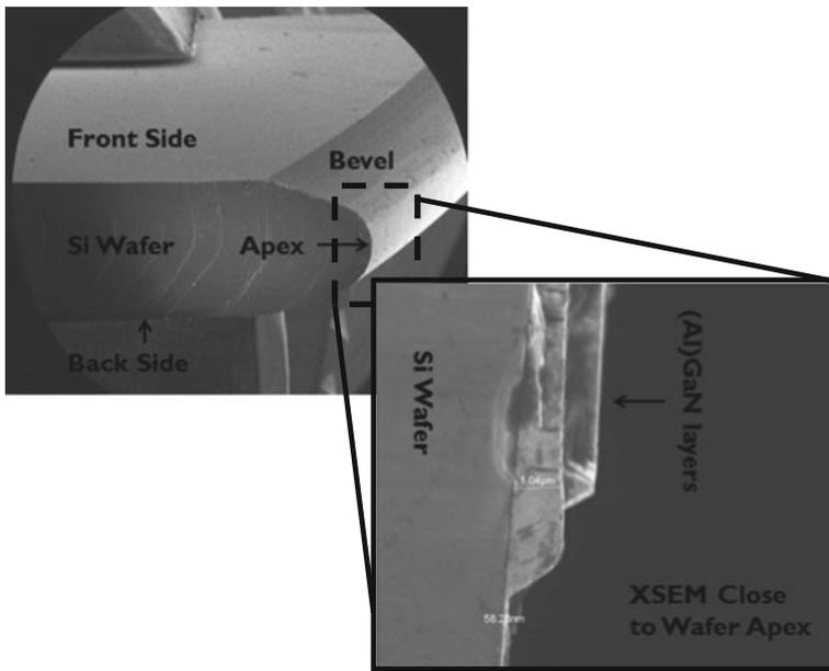
**Fig. 3.17** XSEM analysis of the bevel and backside of a GaN-on-Si substrate after wafer growth. The *inset* shows a magnification of the wafer apex
