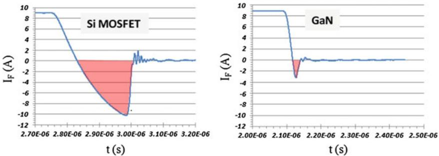
Fig. 10.3 Reverse recovery charge test result for a Si MOSFET and a GaN HEMT with similar on-resistance, showing a 20x reduction in  $Q_{rr}$
