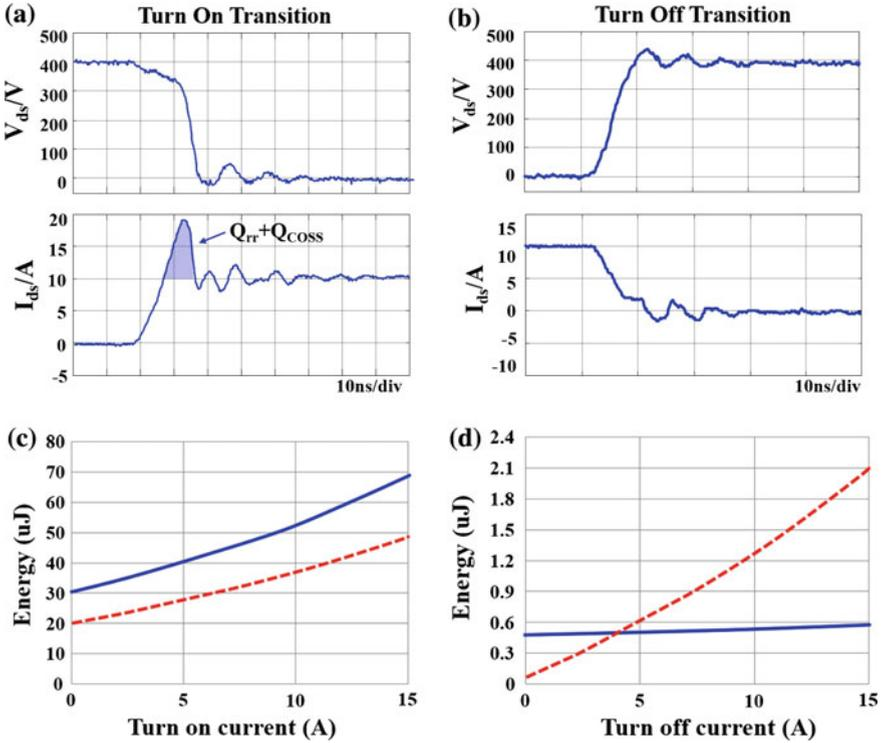
**Fig. 15.1** Switching characteristics of high-voltage GaN switches: **a** Turn-on transition waveforms, **b** turnoff transition waveforms, **c** turn-on switching energy (*solid line* Cascode GaN; *dashed line* e-mode GaN), and **d** turnoff switching energy (*solid line* Cascode GaN; *dashed line* e-mode GaN)
