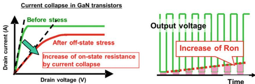
Fig. 11.10 Schematic illustrations to explain Current Collapse of GaN power transistors
