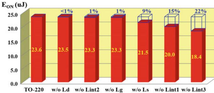
**Fig. 15.4** Device turn-on loss comparison at 400 V/10 A
