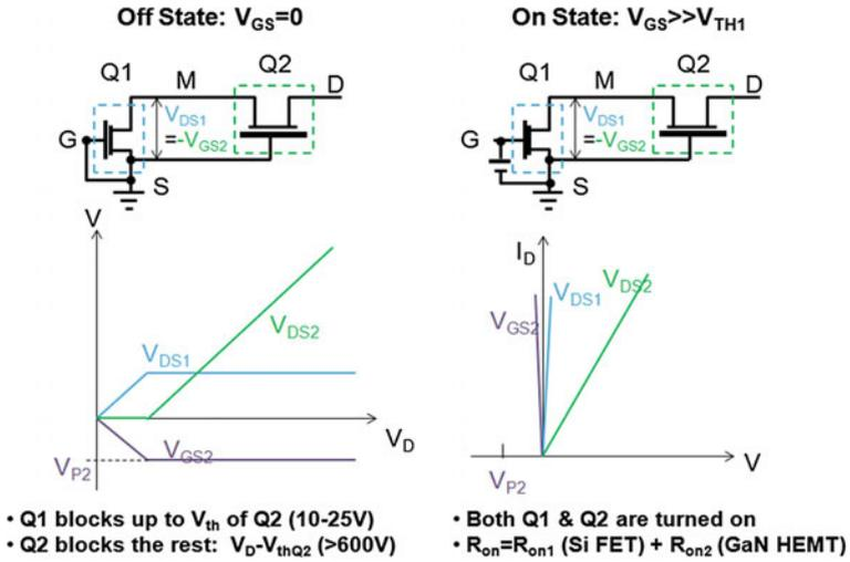
Fig. 10.2 Cascode GaN HEMT off-/on-state operation: Q1 Si FET, Q2 GaN HEMT
