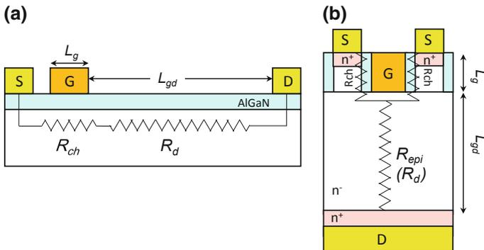
**Fig. 1.20** Schematic illustration of GaN **a** lateral and **b** vertical power devices, where major resistance components are indicated.
