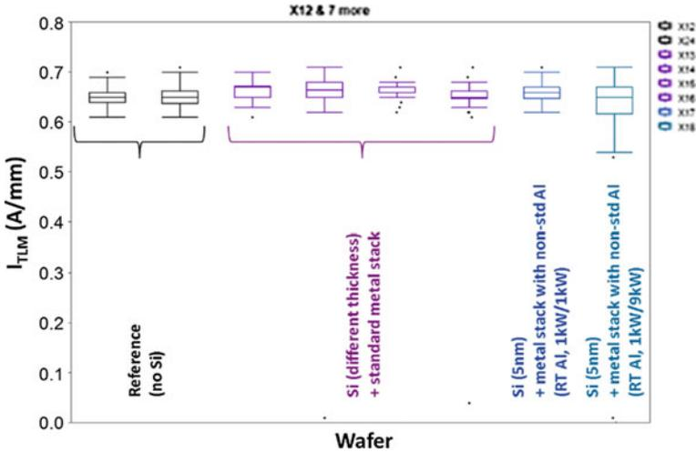
**Fig. 3.15** Saturation current of non-Si- and Si-containing contacts at 10 V between 2 ohmic contacts spaced 12  $\mu\text{m}$
