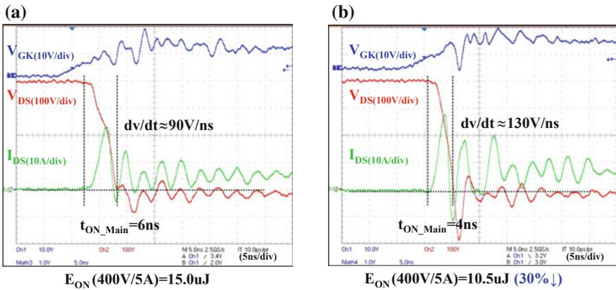
**Fig. 15.6** Turn-on waveform comparison between **a** TO-220 package and **b** stack-die package
