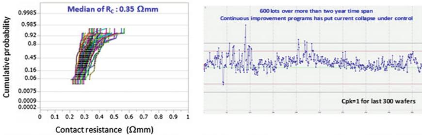
**Fig. 10.15** Example of stringent statistical process control and reproducibility shown by on-wafer resistance distribution and a control chart of dynamic on-resistance across 300 wafers
