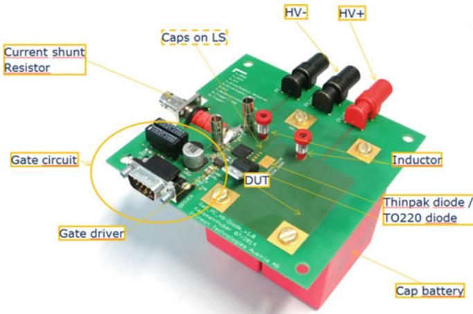
**Fig. 8.13** Inductive load switching application board that has been designed and characterized for normally-off pGaN devices. An integrated asymmetric driving scheme has been used in order to minimize parasitics and to maximize performances
