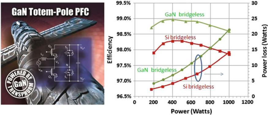
**Fig. 10.7** Totem-pole PFC enabled by diode-free GaN and the resulting performance for a 1-kW application circuit implementation. Higher power 3-kW applications have also been commercialized successfully [10]
