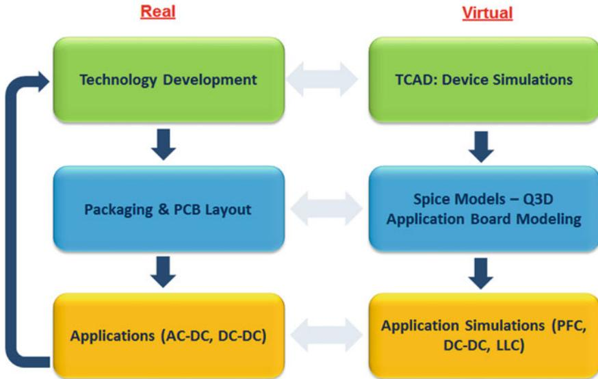
**Fig. 8.1** Schematic view of the GaN virtual prototype approach (VP)
