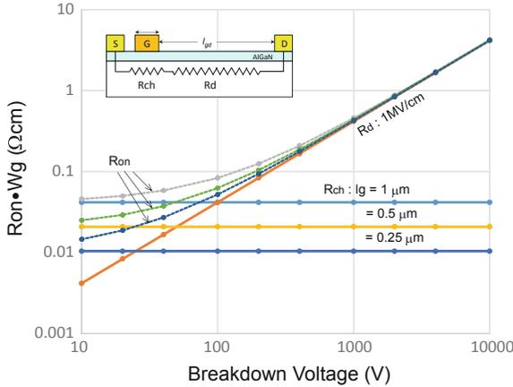
**Fig. 1.14** Calculated  $R_{on} \cdot W_g$  as a function of breakdown voltage for the of typical GaN/AlGaIn FETs with 1.0, 0.5, and 0.25 mm gate length. It is noted that  $R_{on}$  is the sum of  $R_{ch}$  and  $R_d$ . The calculation was done under the conditions of 2DEG mobility of  $1500 \text{ cm}^2/\text{Vs}$  and critical electric field of  $1 \text{ MV/cm}$ , which is a couple of times smaller than the theoretically predicted value
