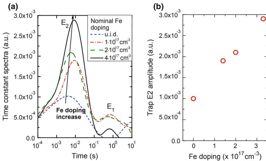
**Fig. 9.6** **a** Time constant spectra measured through drain current transients in devices with iron-doped buffer layer; **b** E2 trap amplitude plotted as a function of iron concentration. Time constant spectra are measured extrapolated from the drain current transient by using the stretched exponential technique
