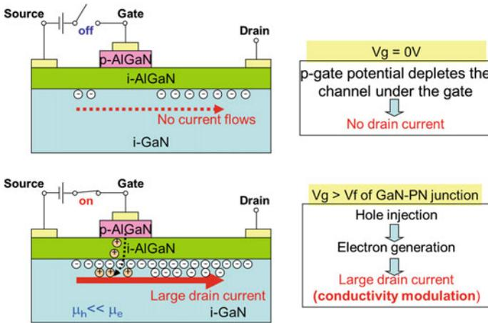
Fig. 11.3 Cross-sectional illustrations describing the operation principle of GIT
