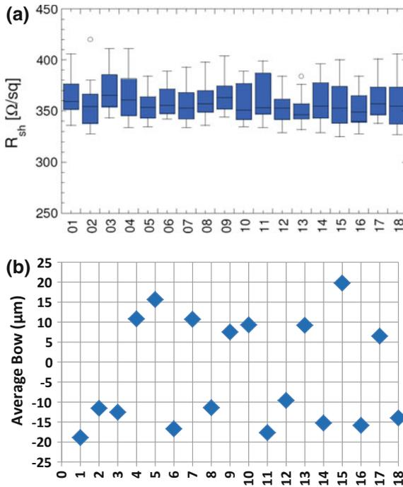
**Fig. 3.2** Reproducibility within a lot of 18,200-mm GaN-on-Si wafers of the (a) 2DEG sheet resistance and (b) wafer bow
