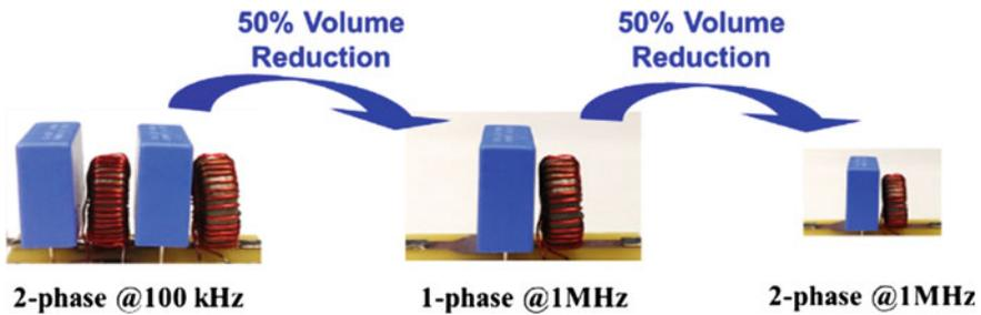
Fig. 15.32 DM filter size comparison
