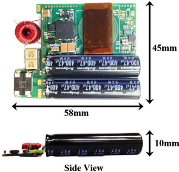
Fig. 15.33 Prototype of MHz flyback converter
