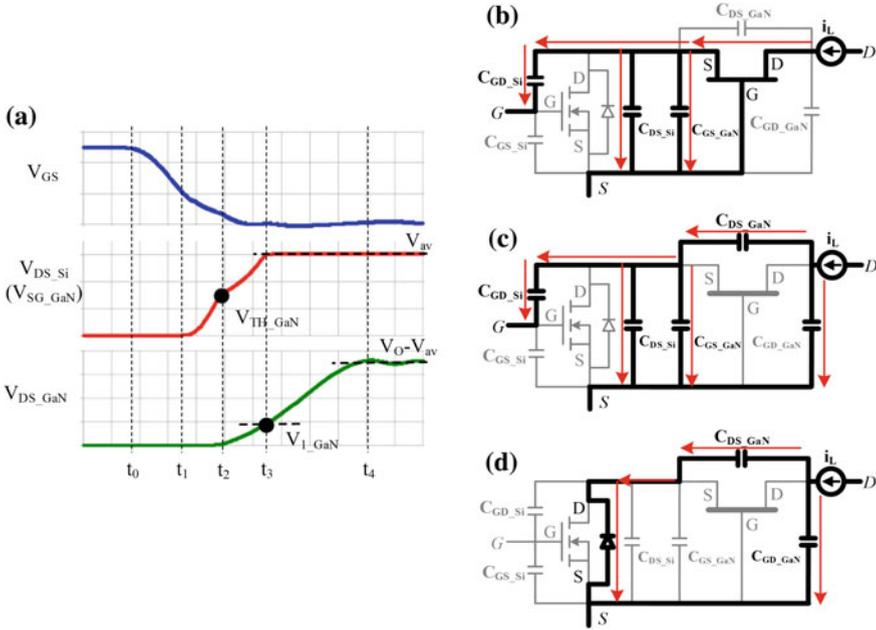
**Fig. 15.11** Voltage distribution of cascode GaN during turnoff transition: **a** Si MOSFET reach avalanche, **b** stage I:  $t_1$ – $t_2$ , **c** stage II:  $t_2$ – $t_3$ , and **d** stage III:  $t_3$ – $t_4$
