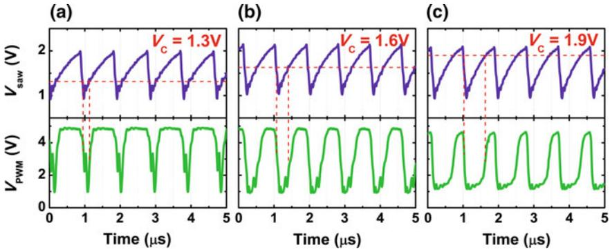
**Fig. 12.24** Waveforms of GaN PWM circuit,  $V_{DD} = 5$  V,  $I_{DD} = 5$  mA.  $V_c$  (red dash) cuts  $V_{saw}$  ( $f = 1.08$  MHz,  $V_{saw} = 0.89$ – $2.18$  V) and determines the duty cycle of  $V_{PWM}$ . **a**  $V_c = 1.3$  V, **b**  $V_c = 1.6$  V, **c**  $V_c = 1.9$  V
