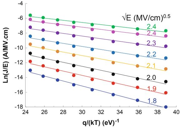
**Fig. 14.16** Extracted activation energy  $E_a$  (see Fig. 14.15) versus  $\sqrt{E}$ . Forward bias condition. Data obtained on capacitor structures
