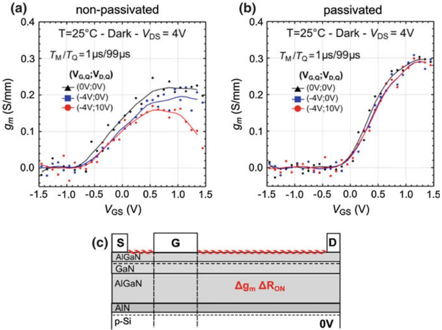
**Fig. 9.4** Pulsed  $g_m$ - $V_G$  measured on **a** non-passivated and **b** passivated HEMTs. When exposed to off-state quiescent bias point, non-passivated devices feature noticeable transconductance peak variation and no  $V_{TH}$  shift
