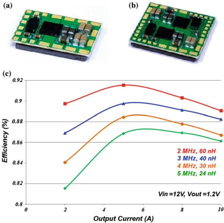
**Fig. 15.25** Three-dimensional integrated POL with IR GaN devices: **a** single-phase version; **b** two-phase version; and **c** efficiency of single-phase version
