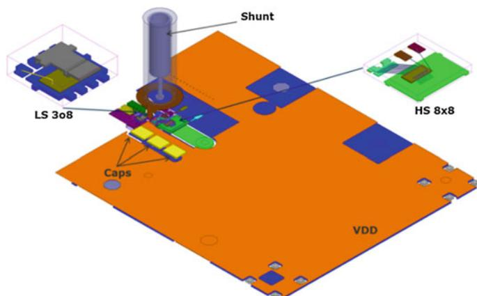
**Fig. 8.21** Application board for the GaN cascode approach
