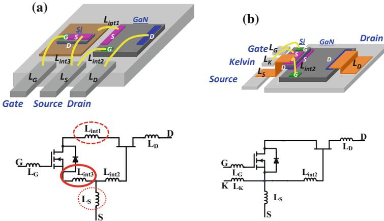
**Fig. 15.5** Package bonding diagram and schematic for cascode GaN HEMT: **a** TO-220 and **b** stack-die
