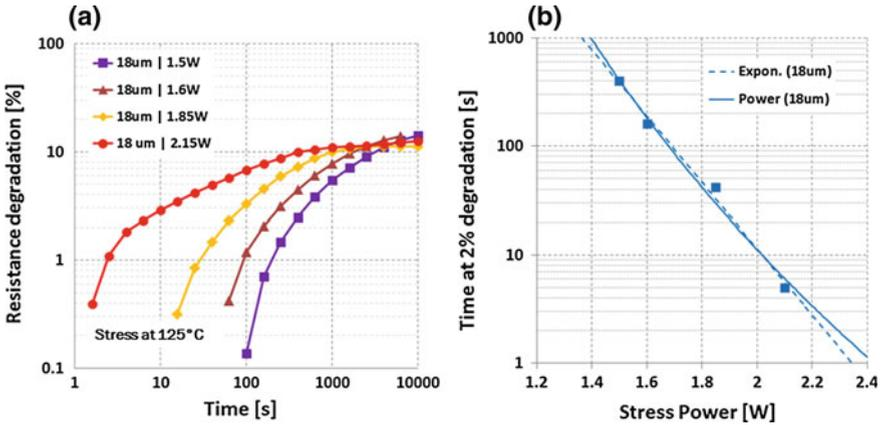
Fig. 14.6 **a** Time evolution of the permanent total resistance degradation as a function of constant power stress measured at 125 °C on 18 μm contact spacing. **b** Time extracted at 2 % degradation as a function of constant stress power. Data are fitted by means of power law (*continuous line*) and of exponential law (*dashed line*)
