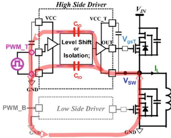
**Fig. 15.20** High  $dv/dt$  deteriorates the PWM signal
