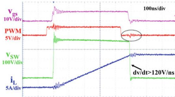
Fig. 15.22 Experimental waveform of improved  $dv/dt$  immunity for high-side driver
