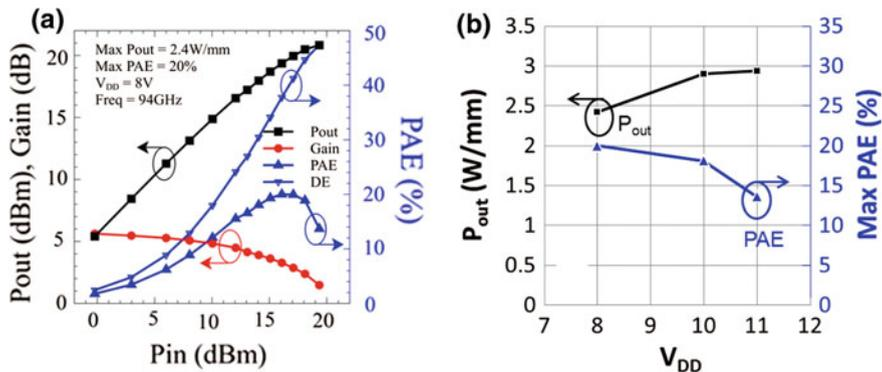
**Fig. 4.14** 94 GHz load pull of N-polar deep recess device with a designed gate length of 75 nm and 110 nm GaN cap passivation in access regions. **a** Power sweep at 8 V bias and **b** maximum power and PAE versus drain bias voltage, falloff in performance is likely related to self-heating [96]
