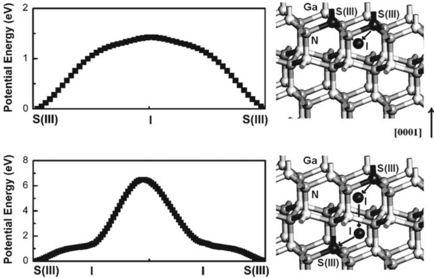
**Fig. 12.7** Potential energy profiles through S(III)-I-S(III) and S(III)-I-I-S(III) paths. The movement paths are shown on the right. The black, dark gray, and light gray balls are F sites, N atoms, and Ga atoms, respectively
