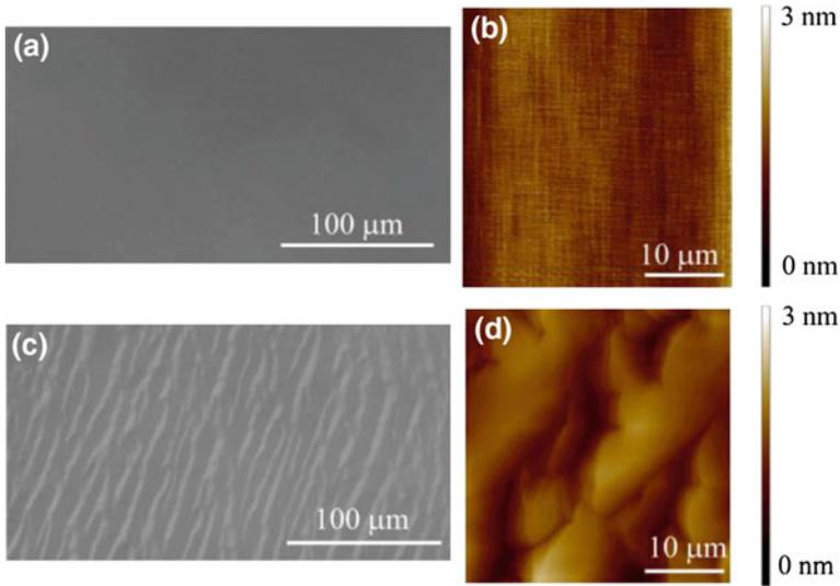
**Fig. 2.11** Normalski images of **a** smooth and **c** rough surface of (Al,Ga)N films grown on bulk GaN substrates, corresponding atomic force microscopy images of **b** smooth and **d** rough surface. Reprinted with permission from Ref. [137]. Copyright 2016, Wiley-VCH Verlag Berlin GmbH, Fed. Rep. of Germany
