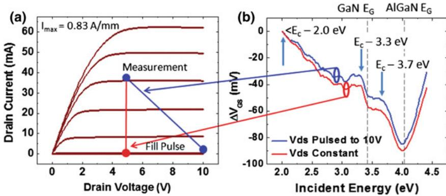
**Fig. 7.10** I-DLOS of an AlGaIn/GaN HEMT without surface passivation. I-DLOS was performed with the device in saturation to probe defects under the gate. The weak dependence of I-DLOS to  $V_{ds}$  for fill pulses with  $V_{gs} < V_{th}$  indicates that defects in the access region do not contribute to the deep-level spectra when the device is biased in saturation. From Ref. [23]
