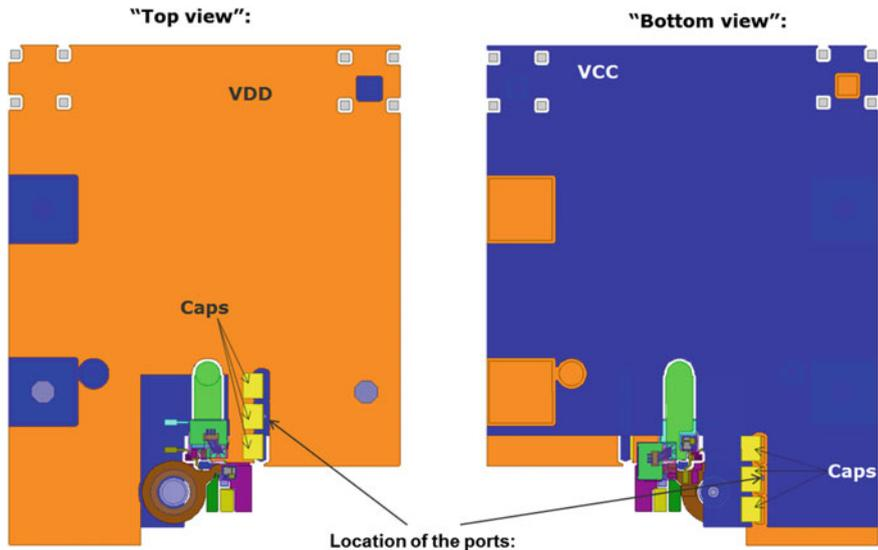
Fig. 8.22 Top view and bottom view of the application board for the GaN cascode approach
