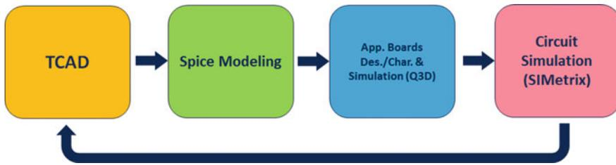
**Fig. 8.15** Schematic description of the GaN Virtual Prototype approach comprising of device simulations, compact model calibration and application board design, characterization and simulation
