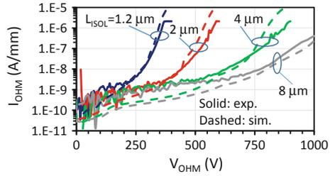
**Fig. 8.11** Experimental (*solid*) and simulated (*dashed*)  $IV$  curves in a vertical, ohmic-to-substrate structure where the voltage  $V_{TOP}$  is applied to the top ohmic contact and the substrate is grounded
