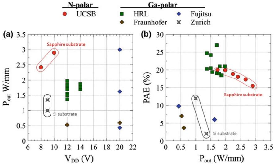
**Fig. 4.5** Summary of reported W-band (75–110 GHz) power device results: **a** output power densities versus drain bias, **b** output power density versus associated power-added efficiency (PAE). Substrate materials are thinned SiC except UCSB which is sapphire, and ETH Zurich which is silicon. Results from UCSB, ETH Zurich, and Fujitsu are load pull, results from HRL Labs and Fraunhofer are matched devices or multi-stage amplifiers [34, 36, 39, 93, 104–115]
