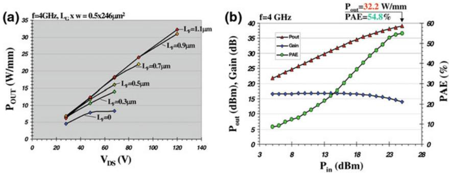
**Fig. 4.3** **a** Output power versus drain bias for different field plates size  $L_F$  shows the effectiveness of field plates in reducing dispersion at high drain bias, **b** power sweep for largest field plate shows record breaking 32.2 W/mm power density [11]
