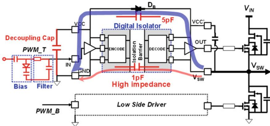
Fig. 15.21 Simplified high-side driving circuit
