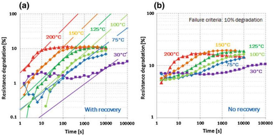
**Fig. 14.8** Time evolution of the total resistance degradation as a function of chuck temperature for 6  $\mu\text{m}$  contact spacing stressed at a constant power of 1.25 W **a** permanent degradation, i.e., after recovery; **b** immediately after stress, i.e., without recovery
