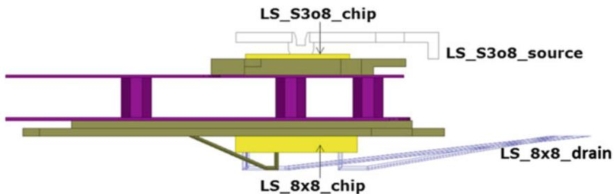
Fig. 8.23 Front view of the application board for the GaN cascode approach with emphasis on the low-side cascade. The GaN HEMT and the LV MOSFET are mounted on the opposite sides of the PCB
