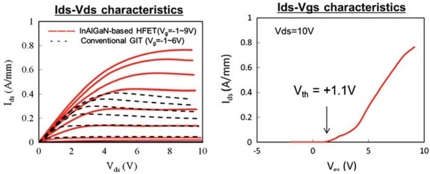
**Fig. 11.22**  $I_{ds}$ - $V_{ds}$  and  $I_{ds}$ - $V_{gs}$  characteristics of the GIT fabricated over InAlGaN/GaN, where  $I_{ds}$ - $V_{ds}$  of the conventional GIT on AlGaN/GaN is also shown
