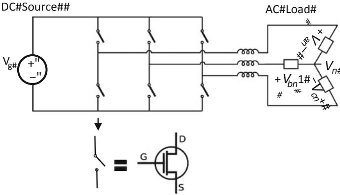
**Fig. 5.1** A 3-phase inverter circuit showing conversion of DC to 3-phase AC signal. The switches represented in the figure schematically are transistors in a solid-state power converter
