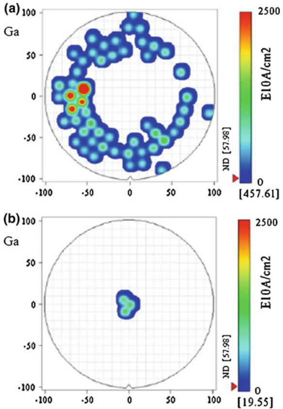
**Fig. 3.20** Monitoring of Ga contamination on 3 etching tools during three loops of GaN-on-Si wafers processing. The contamination of each tool without special cleaning procedure is also reported. The maximum allowed contamination level is indicated in the figure
