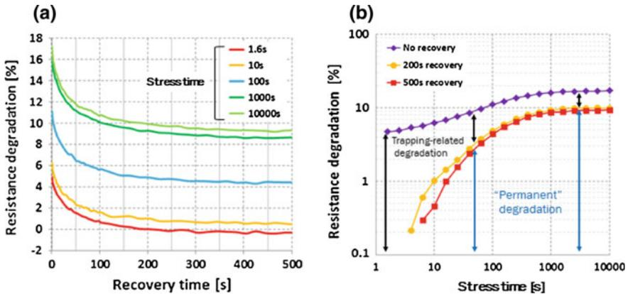
**Fig. 14.4** **a** Time evolution of the total resistance during recovery time as a function of stress step time during 1.25 W constant power stress. **b** Corresponding time evolution of the total resistance during stress time as a function of recovery time (at 125 °C for 6  $\mu\text{m}$  contact spacing)
