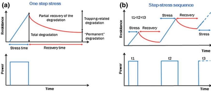
Fig. 14.3 Schematic of resistance and power evolution to access the “permanent” degradation. **a** One step stress and recovery sequence; **b** Multiple sequences step stress and recovery sequences
