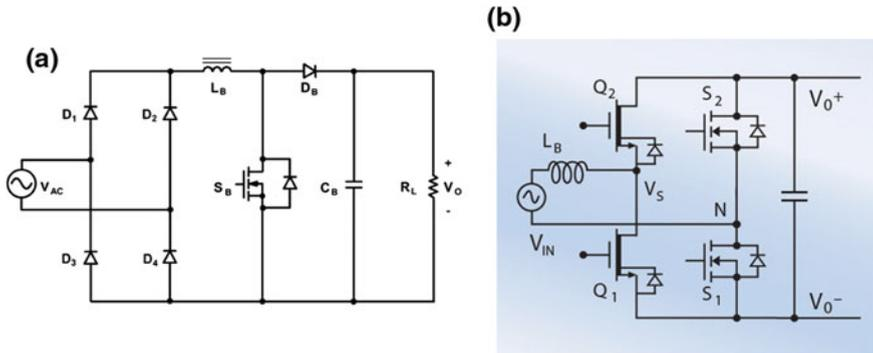
**Fig. 4.25** **a** Traditional PFC with line rectifying bridge, and **b** totem pole PFC with no diode drop,  $Q_1$  and  $Q_2$  are fast PWM switches, and  $S_1$  and  $S_2$  are 60 Hz slow switches. The low reverse recovery charge ( $Q_{rr}$ ) and bidirectional capability of GaN enable this bridgeless PFC
