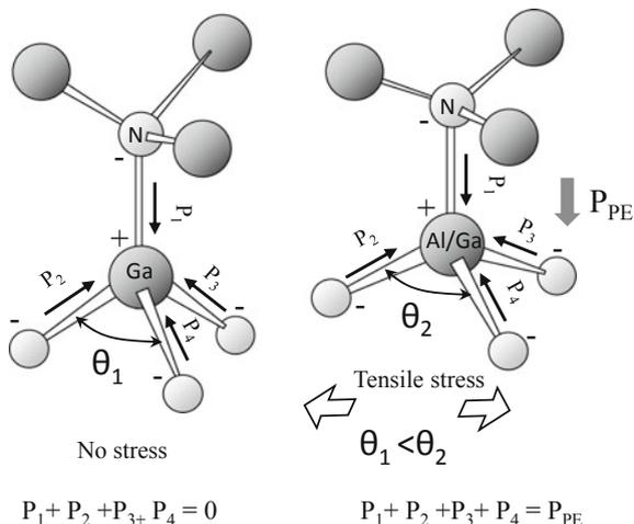
**Fig. 1.5** The balanced polarization of ionic bonds in the tetrahedron shape (*left*) cause the unbalance of polarization field under the stress originated to the difference of lattice constant of underlying material. The resultant electric field is called piezo electric one, shown as  $E_p$  in the figure (*right*)
