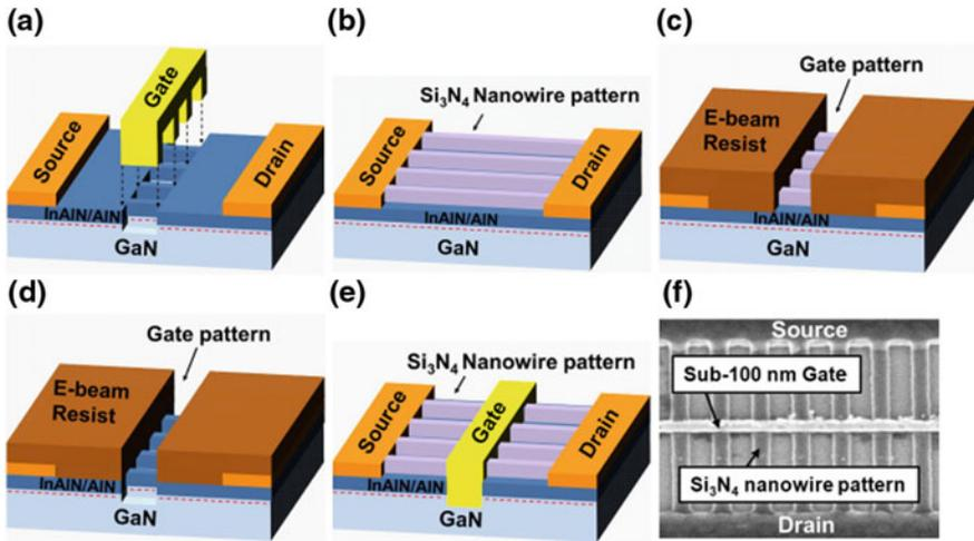
**Fig. 6.10** a Device structure of nanowire channel HEMT, b  $\text{Si}_3\text{N}_4$  nanowire pattern, c gate patterning and channel etching, d  $\text{Si}_3\text{N}_4$  removal, e gate lift off, f SEM image after gate. Adapted from [48]
