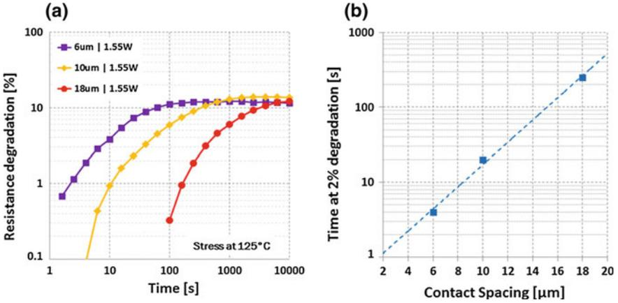
Fig. 14.5 **a** Time evolution of the permanent total resistance degradation during 1.55 W constant power stress at 125 °C for 6, 10, and 18 μm contact spacings. **b** Time extracted at 2 % degradation as a function of contact spacing
