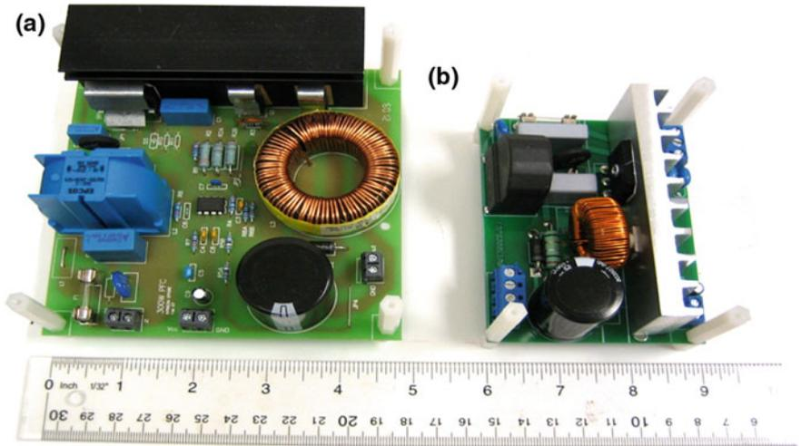
Fig. 4.23 Comparison of comparable PFC circuits: **a** silicon-based, requiring a two stage EMI filter and large inductors, and **b** GaN-based with smaller inductor size, one less EMI filter stage, enabled by the lower-loss transistors and diodes
