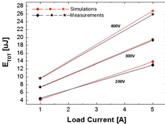
**Fig. 8.26** Total switching energy of the normally-off pGaN transistor. Comparison between measurements and simulations is shown
