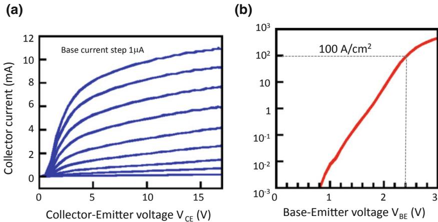
**Fig. 1.25** **a** Obtained I-V characteristics of GaN/InGaN DHBT, where hfe over 1000 is seen, **b** obtained collector current density as a function of base-emitter voltage ( $V_{BE}$ ), where current handling capability over 100 A/cmm<sup>2</sup> is seen [28]
