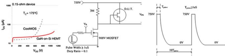
**Fig. 10.14** 600 V GaN HEMT with low leakage and  $V_{bd} > 1000$  V along with a standard spike rating of 750 V
