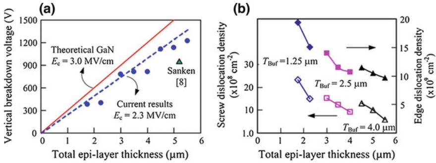
**Fig. 2.4** **a** Vertical breakdown voltage as a function of the total epilayer thickness. **b** Screw (*hollow symbols*) and edge (*solid symbols*) dislocation densities derived from XRD measurements for (Al,Ga)N epitaxial layers grown on Si with various total thicknesses. Reprinted with permission from Ref. [56]. Copyright 2011, IEEE
