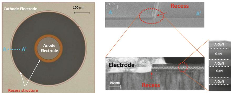
**Fig. 1.11** Chip photo micrograph of fabricated NSJ diode with SEM cross section of the three layer structure. It is noted that Ti/Al and Pt/Au were used for cathode and anode, respectively
