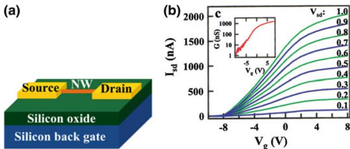
**Fig. 6.1** **a** Schematic of a NW FET. **b**  $I$ - $V_g$  data for values of  $V_{\text{sd}} = 0.1$ – $1$  V. *Inset* Conductance  $C$  versus gate voltage. Reprinted with permission from [26]—copyright 2016 American Chemical Society
