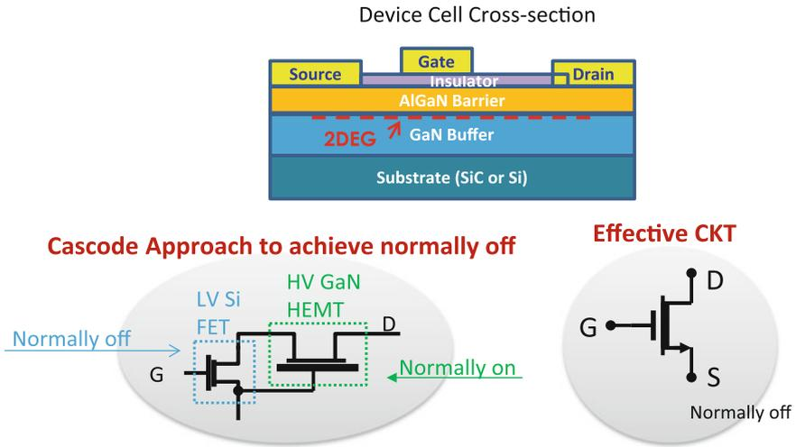
**Fig. 4.17** Cascode method for normally off operation. Disadvantage: two chips required
