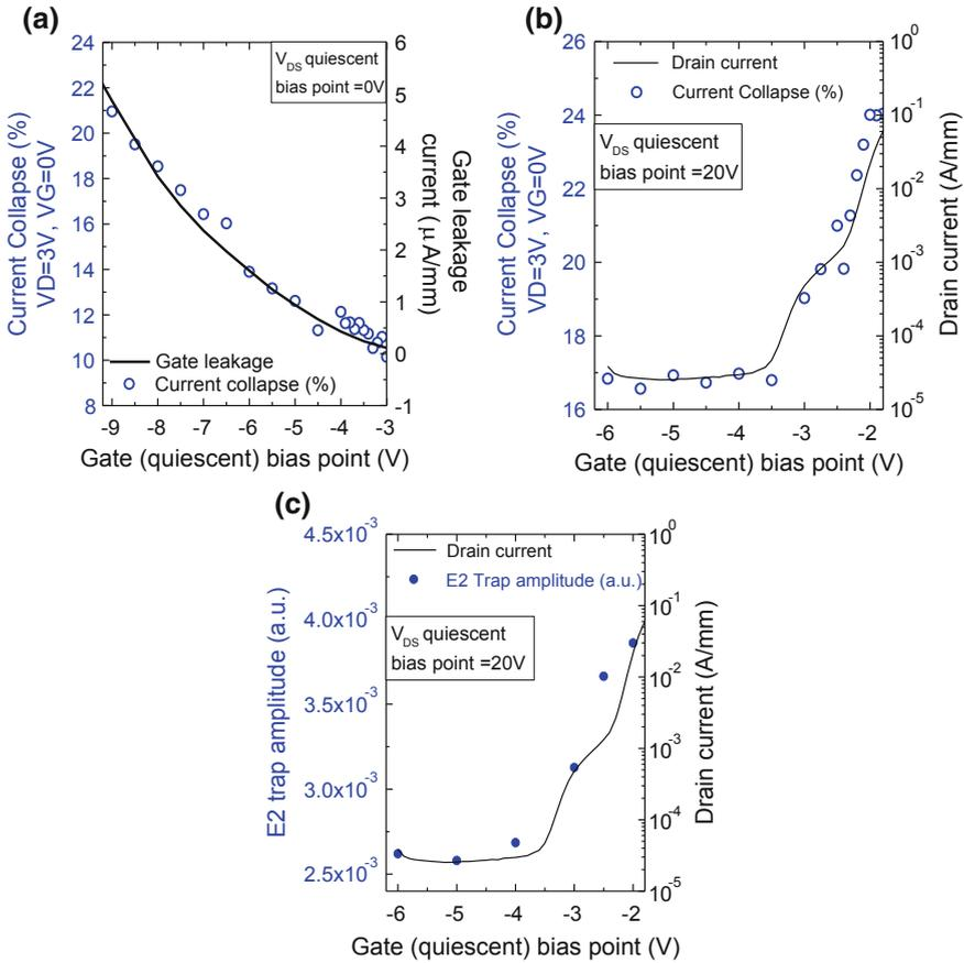
**Fig. 9.8** Dependence between the dynamic performance of devices with iron doping buffer compensation and the leakage current measured in off state (a) or the drain current evaluated in off and semi-on state (b). Enhancement of the trap E2 signal measured in off and in semi-on state (c). The current collapse is defined as the ratio of the current variation in two quiescent bias points to the current measured in the first one
