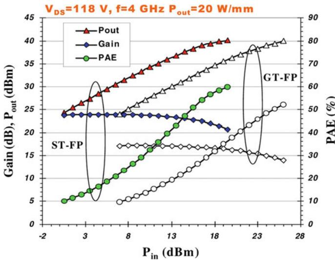
**Fig. 4.4** Power sweep of source terminated field plate (ST-FP) and gate terminated (GT-FP) shows the tradeoff between the two field plate designs, with higher gain from ST-FP due to reduced gate drain capacitance with this approach [12, 13]
