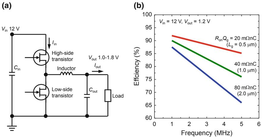
Fig. 1.18 a Half-bridge circuit to make DC-to-DC converter and b obtained conversion efficiency as a function of switching frequency for devices with three different  $R_{on} \cdot Q_g$
