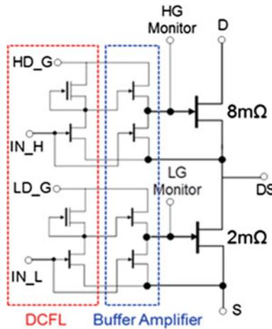
**Fig. 11.23** Circuit diagram of the DC-DC converter (POL) IC with gate drivers
