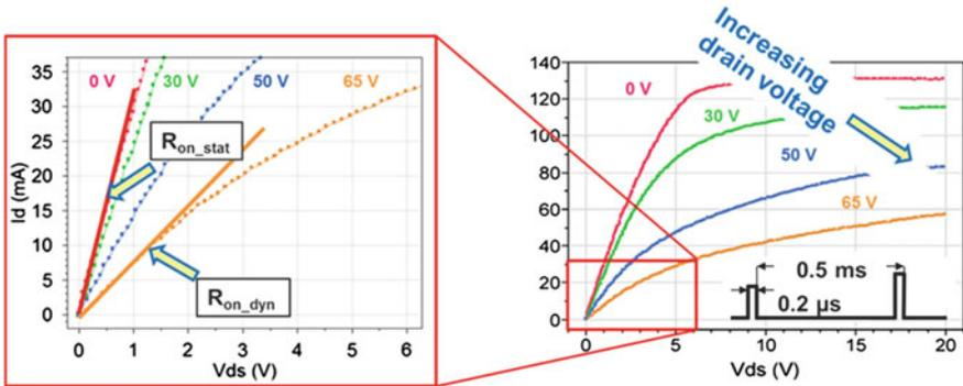
**Fig. 13.3** Increase of dynamic on-state resistance upon device switching from a high drain voltage off-state bias point to any point of the output IV-characteristics, see also [16]
