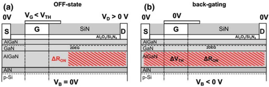
**Fig. 9.16** **a** In the off state, the dominant charge-trapping mechanism is promoted by vertical drain-to-substrate potential, is localized in the gate–drain access region within the epitaxial buffer/back-barrier layers, and causes the dynamic  $R_{ON}$  increase. **b** In back-gating stress, charge trapping affects the entire source-to-drain length, promoting not only the dynamic  $R_{ON}$  increase, but also the shift of the threshold voltage
