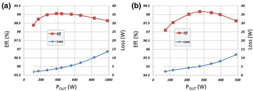
**Fig. 4.26** Efficiency of bridgeless GaN totem pole PFC versus output power, at 50 kHz switching frequency and 390 V output voltage for **a** 230 V input and **b** 115 V input
