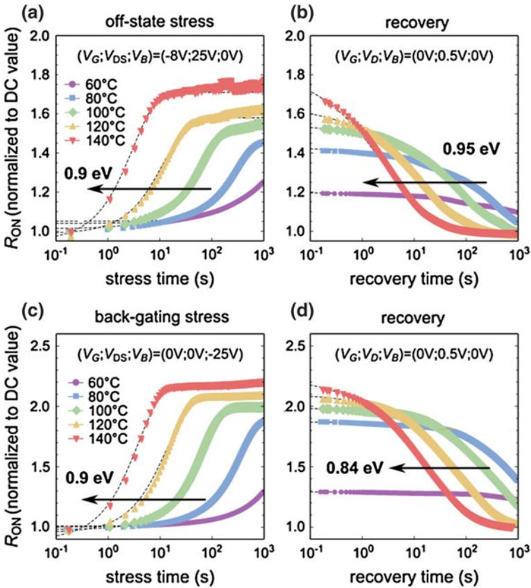
**Fig. 9.15** Stress and recovery transients performed in off-state and back-gating stress. Both charge trapping and charge detrapping are thermally activated. Off-state stress and back-gating stress lead to similar stress/recovery transients, suggesting unique charge-trapping mechanism localized in the buffer. Data from Bisi et al. [98]
