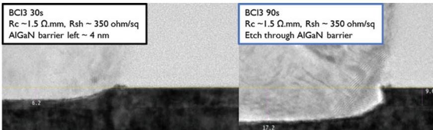
Fig. 3.11 TEM on ohmic regions with  $R_C$  of  $\sim 1.5 \Omega \text{ mm}$
