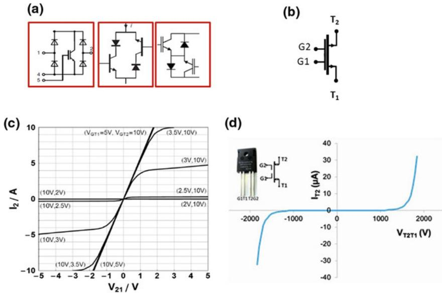
**Fig. 4.27** **a** Typical silicon-transistor implementations of a four-quadrant switch (FQS), requiring 4 or 5 devices, **b** schematic of a GaN FQS, incorporating the same functionality in a single device, **c** on-state and **d** off-state  $I-V$  characteristics of the GaN FQS showing capability for low on-resistance and high current and voltage blocking in both directions
