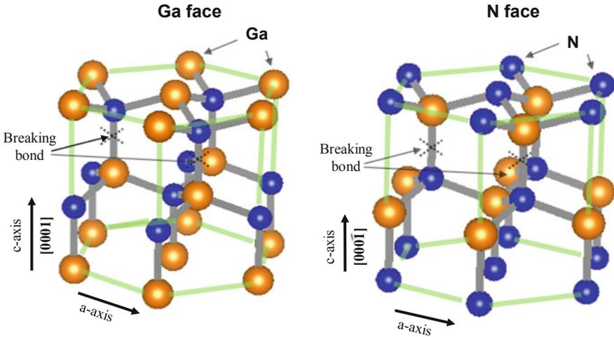
**Fig. 1.4** Asymmetrical hexagonal GaN crystal structure along  $c$ -axis, where either Ga- or N-face appears at the surface of the crystal
