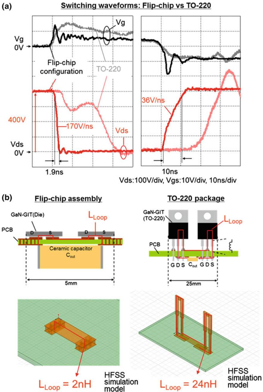
**Fig. 11.9** Switching waveforms of GITs with **a** flip-chip assembly and **b** TO-220 packaging, where the simulation results on parasitic inductances are also shown
