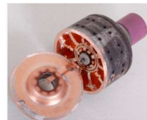
Major elements of the magnetron.
