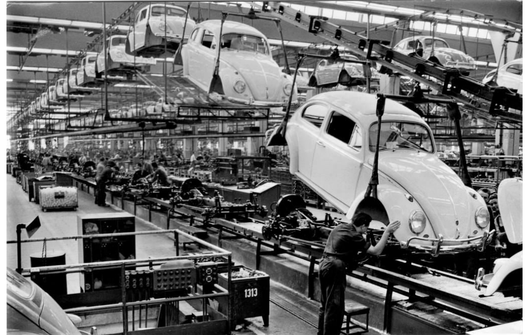
Volkswagen Beetle Assembly Line (By Alden Jewell , license: CC BY 2.0 )
