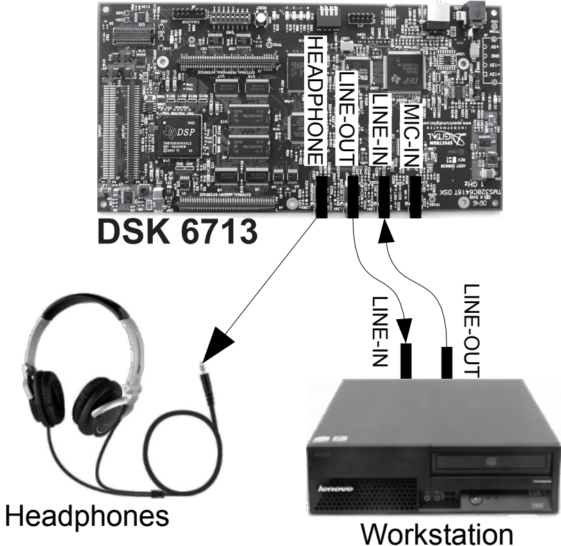
Figure 4: Set-up for evaluating digital audio algorithms using the DSK6713
