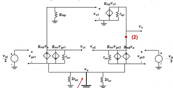
One can also get the correct results by assuming a-priori that the in the difference-mode the voltage  $v_s$  is approximately zero (i.e. the node is a small signal ground)
