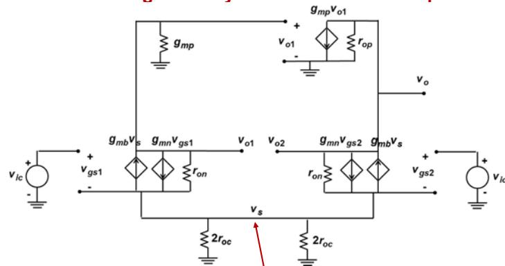
So one can assume that in the common-mode, even with the current mirror, no current flows in the bottom most horizontal wire (i.e. it is a small signal open)
