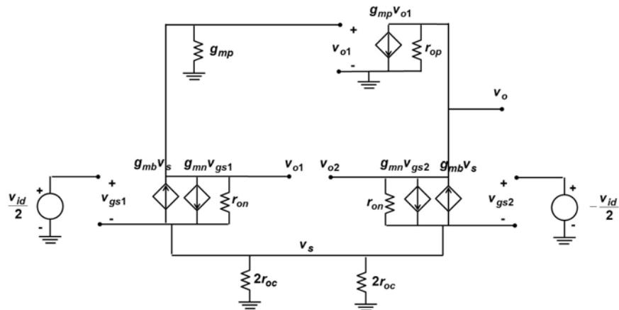
There are three unknown internal voltage variables:  $v_{o1}$   $v_{o2}$   $v_s$
