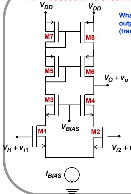
What if one needs a large gain and a large output resistance from a differential (transconductance) amplifier?
