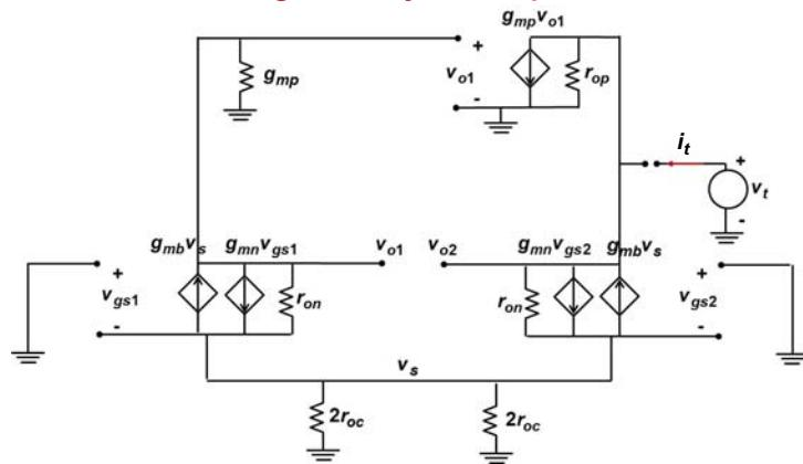
$$R_{out} \approx r_{on} \parallel r_{op}$$
