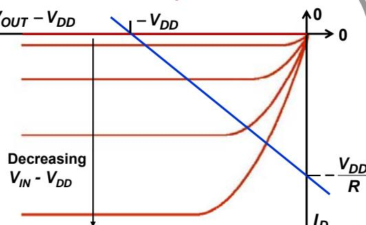
$$I_D = \begin{cases} 0 & \text{For } V_{IN} - V_{DD} > V_{TP} \\ -k_p \left[ V_{IN} - V_{DD} - V_{TP} - \frac{V_{OUT} - V_{DD}}{2} \right] (V_{OUT} - V_{DD}) & \text{For } 0 \geq V_{OUT} - V_{DD} \geq V_{IN} - V_{DD} - V_{TP} \\ -\frac{k_p}{2} (V_{IN} - V_{DD} - V_{TP})^2 & \text{For } 0 \geq V_{IN} - V_{DD} - V_{TP} \geq V_{OUT} - V_{DD} \end{cases}$$
