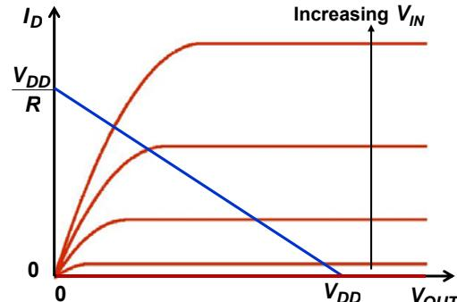
$$I_D = \begin{cases} 0 & \text{For } V_{IN} < V_{TN} \\ k_n \left[ V_{IN} - V_{TN} - \frac{V_{OUT}}{2} \right] V_{OUT} & \text{For } 0 \leq V_{OUT} \leq V_{IN} - V_{TN} \\ \frac{k_n}{2} (V_{IN} - V_{TN})^2 & \text{For } 0 \leq V_{IN} - V_{TN} \leq V_{OUT} \end{cases}$$
