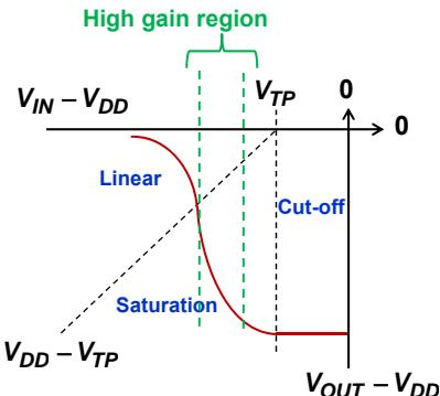
In the high gain region, the slope  $\left| \frac{dV_{OUT}}{dV_{IN}} \right|$  can be larger than unity!
