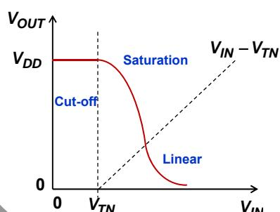
A high input voltage produces a low output voltage
