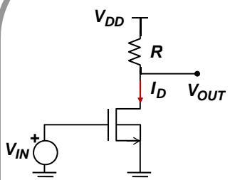
$$I_D = k_n \left[ V_{IN} - V_{TN} - \frac{V_{OUT}}{2} \right] V_{OUT}$$
