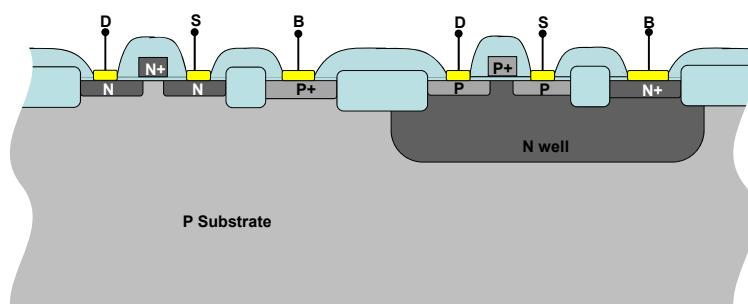
The NFETs and the PFETs can be realized on the same P-substrate by making a N-well inside the substrate for the PFETs
