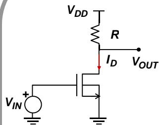
$$I_D = \frac{V_{DD} - V_{OUT}}{R}$$
