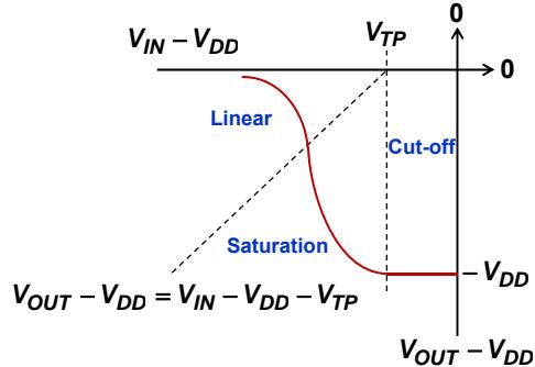
A high input voltage produces a low output voltage
