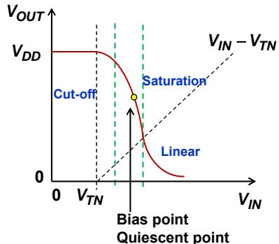
What is:  $\frac{V_{out}}{V_{in}} = ?$  → Voltage gain
