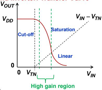
In the high gain region, the slope  $\left| \frac{dV_{OUT}}{dV_{IN}} \right|$  can be much larger than unity!
