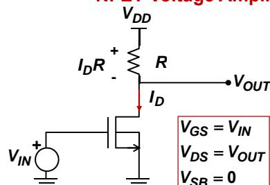
We need to find the relation between the output and the input voltage
