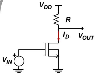
$$I_D = \frac{k_n}{2} (V_{IN} - V_{TN})^2$$
