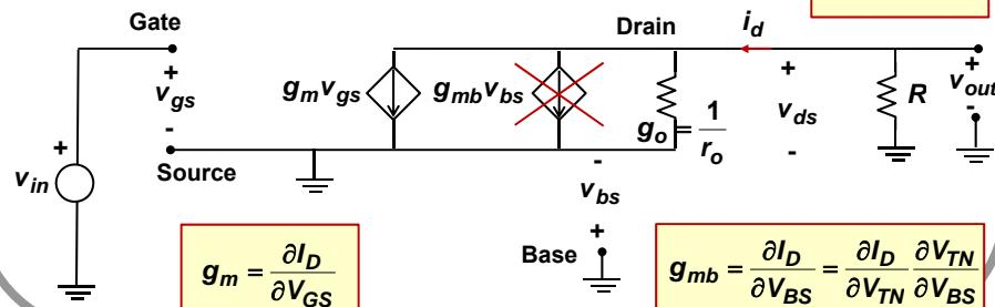
$$g_m = \frac{\partial I_D}{\partial V_{GS}}$$
