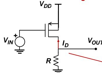
We need to find the relation between the output and the input voltage
