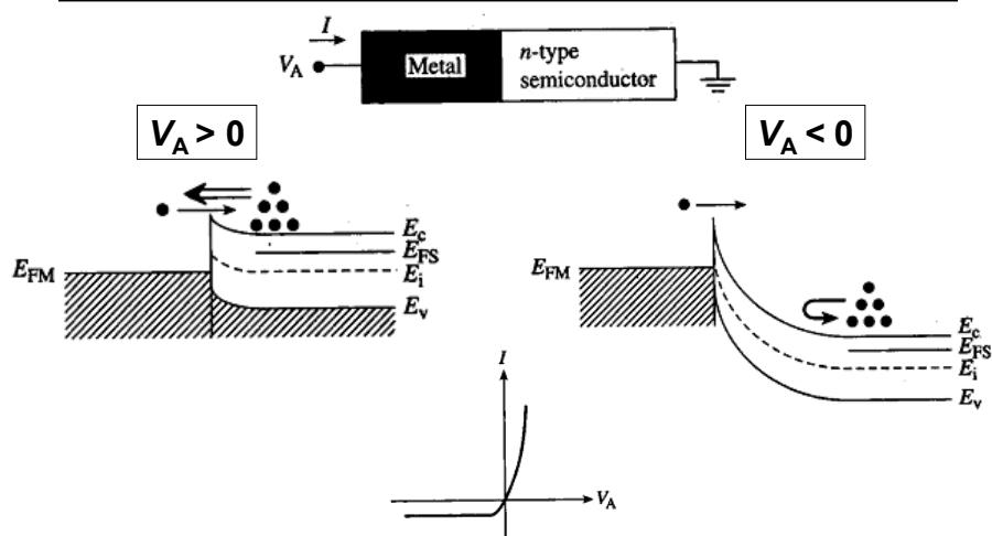
Fermi level splits into two levels ( $E_{FM}$  and  $E_{FS}$ ) separated by  $qV_A$
