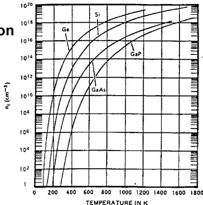
$$Si: \quad n_i = 3.9 \times 10^{16} T^{3/2} e^{-\frac{0.605 \text{ eV}}{kT}} / \text{cm}^3$$
