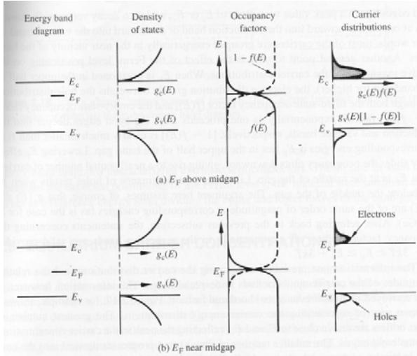
$$\begin{aligned} n &= n_i e^{(E_F - E_i)/kT} \\ &= N_c e^{(E_c - E_F)/kT} \end{aligned}$$
