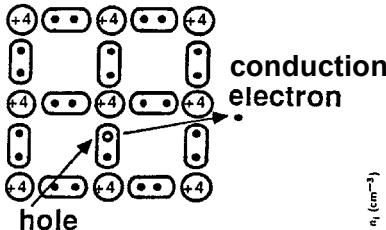
Covalent (shared  $e^-$ ) bonds exists between Si atoms in a crystal. Since the  $e^-$  are loosely bound, some will be free at any T, creating hole electron pairs.
