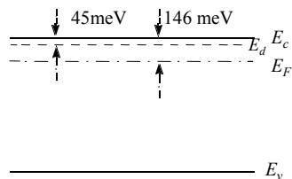
$$\text{Probability of non-ionization} \approx \frac{1}{1 + e^{(E_d - E_F)/kT}} = \frac{1}{1 + e^{((146-45)\text{meV})/26\text{meV}}} = 0.02$$
