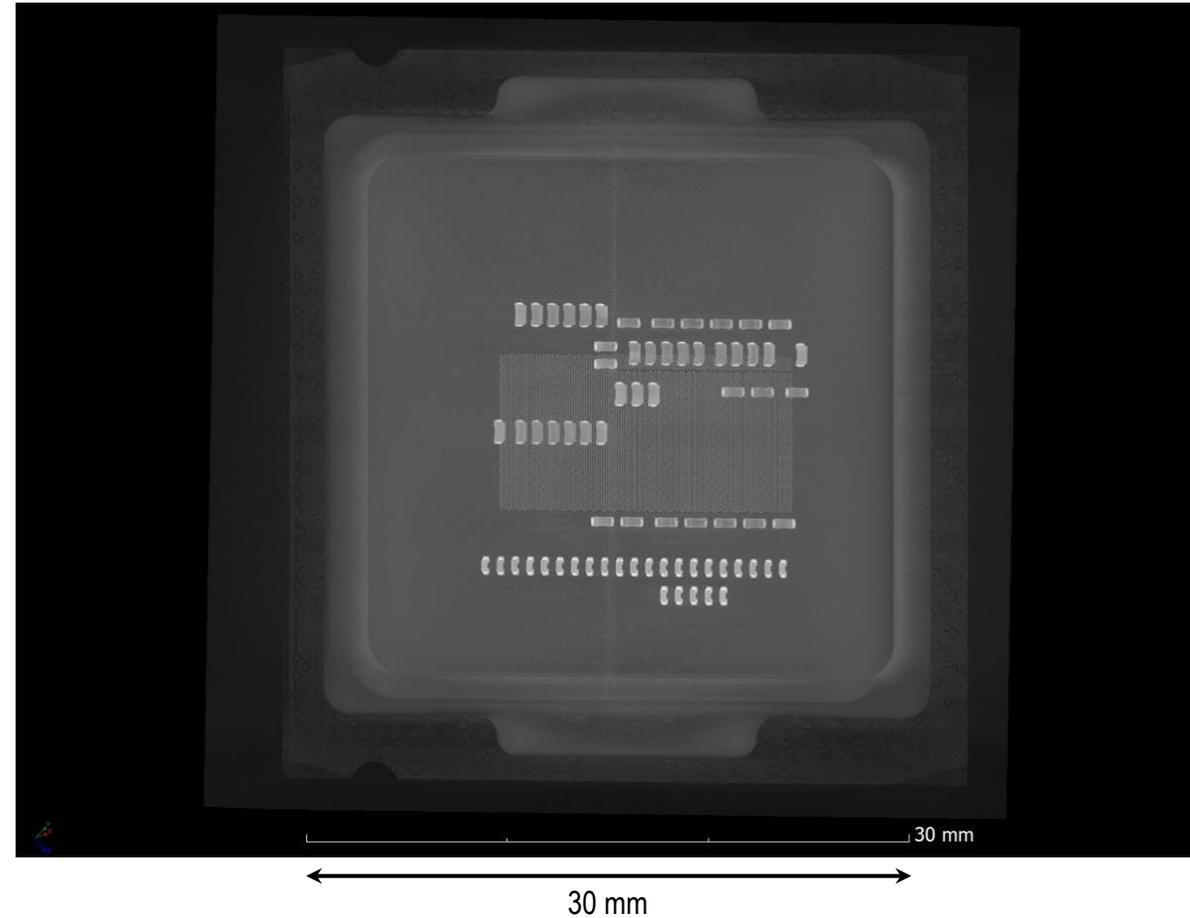
3D volume rendering ( $18 \mu\text{m}^3$  voxels) of flip-chip area, Intel G3260 microprocessor ID 0402
