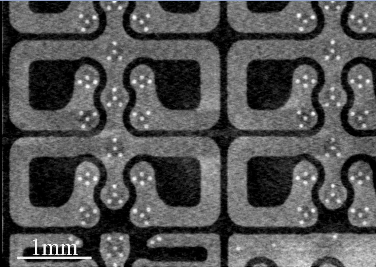
3D volume rendering ( $6 \mu\text{m}^3$  voxels) of Intel G3260 processor flip-chip area
