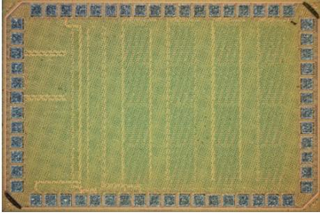
USC-designed digitizing matrix-multiplier chip for ML manufactured by Global Foundries in 2017 in 14nm FinFET CMOS technology
