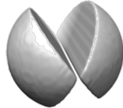
Missing *wedge* in 3D diffraction data
