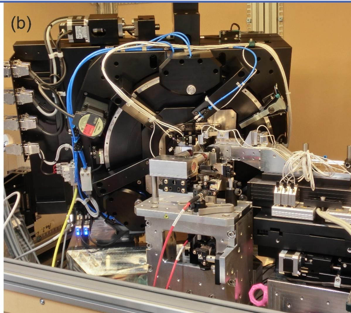
Laminography microscope at SLS cSAXS beamline with enclosure doors removed. (a) Overview with flight tube and control rack. (b) Stage detail
