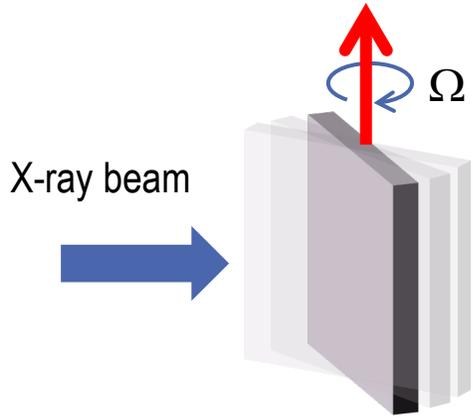
Limited-angle tomography at normal incidence ( $\theta=90^\circ$ ) and limited rotation  $W$  about chip-plane
