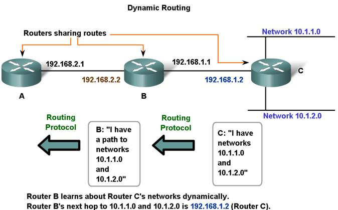
Router A learns about Router C's networks dynamically from Router B. Router A's next hop to 10.1.1.0 and 10.1.2.0 is 192.168.2.2 (Router B).
