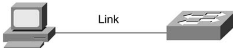
Figure 8-1. Example Point-to-Point Interconnection
