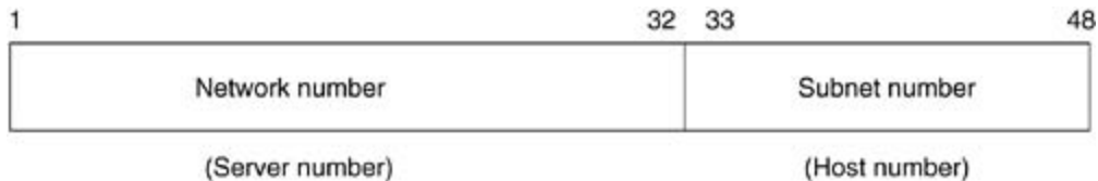
Figure B-7. A VINES Address Consists of a Network Number and a Subnet Number
