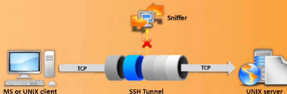
FIGURE 19.7: Secure shell tunneling
