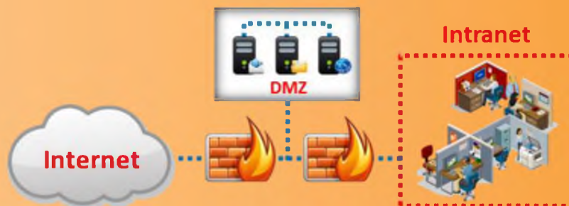
FIGURE 17.7: Multi-Homed Firewall Architecture
