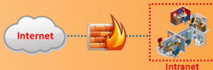
FIGURE 17.5: Bastion Host Architecture
