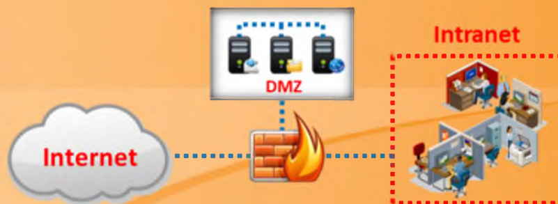
FIGURE 17.6: Screened Subnet Architecture
