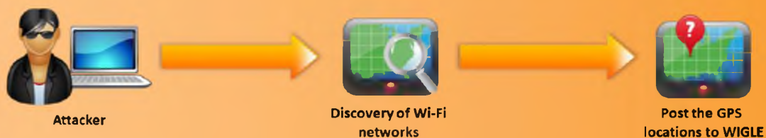
FIGURE 15.36: Tracking the location of the discovered Wi-Fi network and uploading it to WIGLE site
