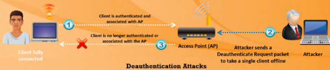
FIGURE 15.52: Attacker performing deauthentication attack on client system
