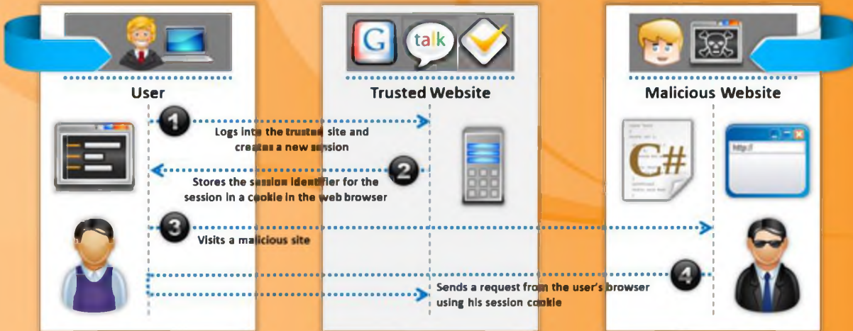
FIGURE 13.23: Cross-site Request Forgery (CSRF) Attack
