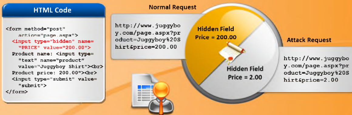
FIGURE 13.14: Hidden Field Manipulation Attack
