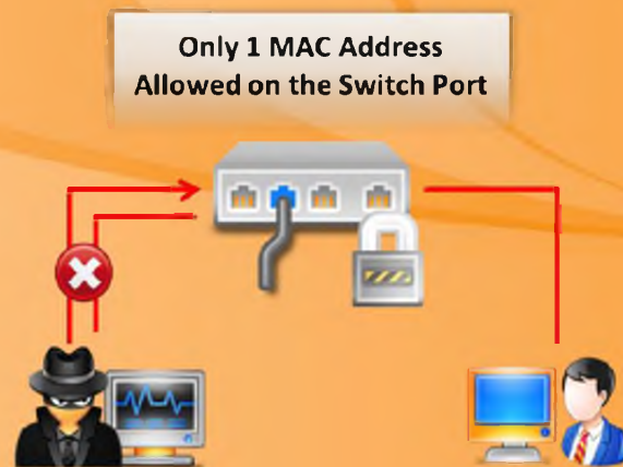
FIGURE 8.21: User Protection from MAC Flooding
