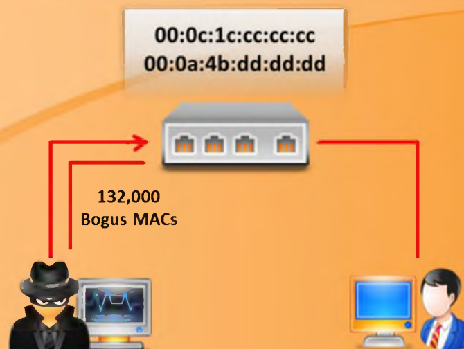
FIGURE 8.20: Attacker Flooded the Switch with Fake Make Address
