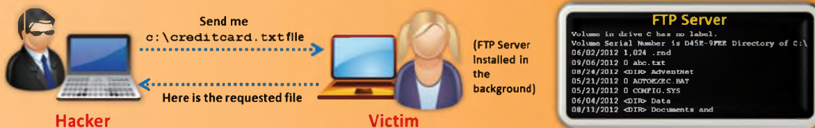
FIGURE 6.21: Attacker infecting victim's system using FTP Trojans
