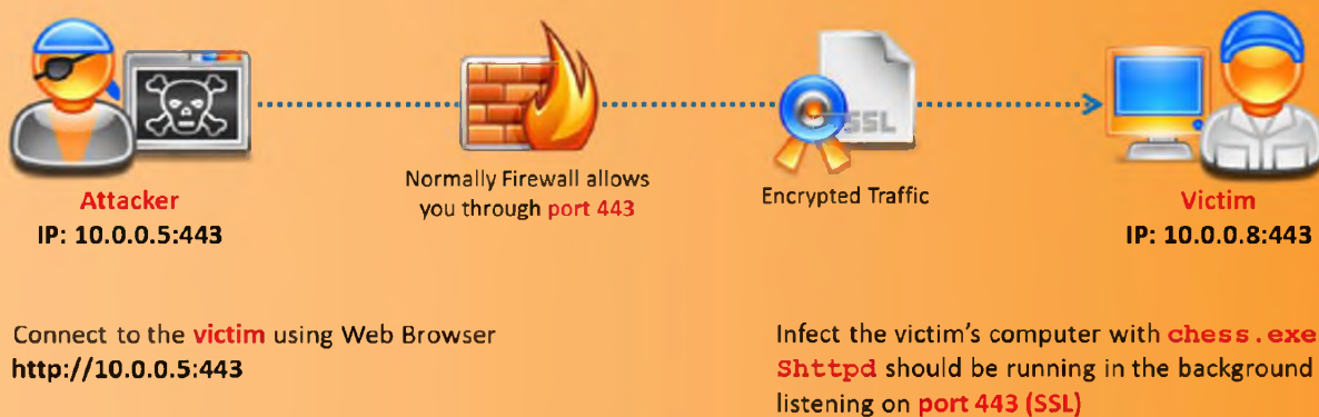
FIGURE 6.26: Attacker infecting Victim's system using Sshhttpd Trojan
