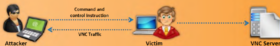
FIGURE 6.23: Attacker uses victim's computer as VNC server using VNC Trojans
