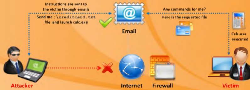
FIGURE 6.15: Illustrating the attack process using email Trojans
