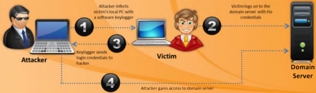
FIGURE 5.12: Stealing Passwords Using Keyloggers
