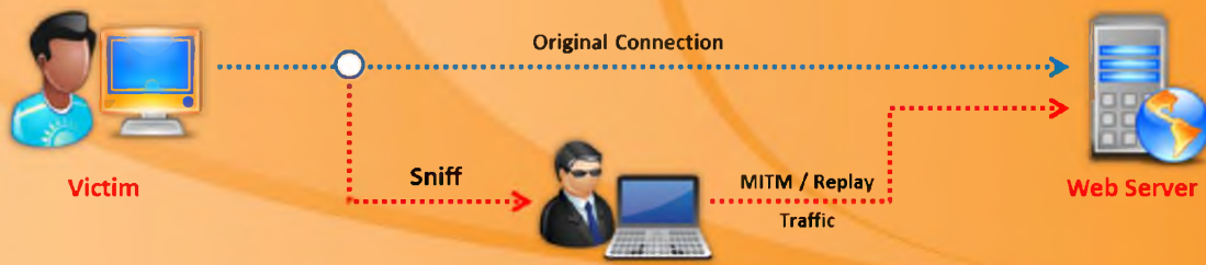
FIGURE 5.4: Passive Online Attack by Using Man-in-the-Middle and Replay Attack
