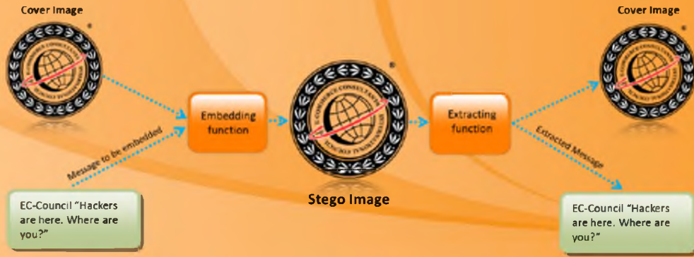
FIGURE 5.65: How Steganography Works
