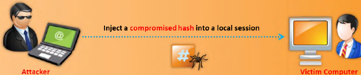
FIGURE 5.6: Active Online Attack by Using Hash Injection Attack
