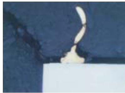
Cracks on the package top surface (wire disconnection with electrical effects)
