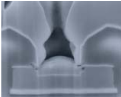
Figure 4.2 Al Wiring Coverage Disconnection
