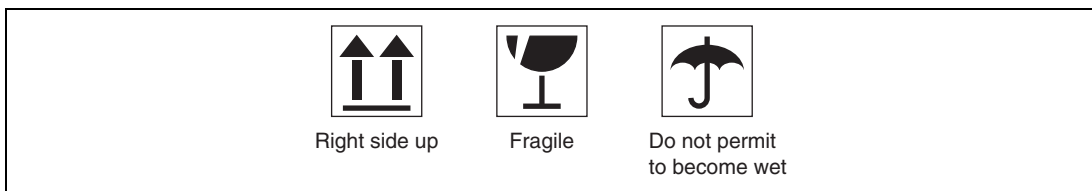
Figure 6.23 Examples of Exterior Labeling
