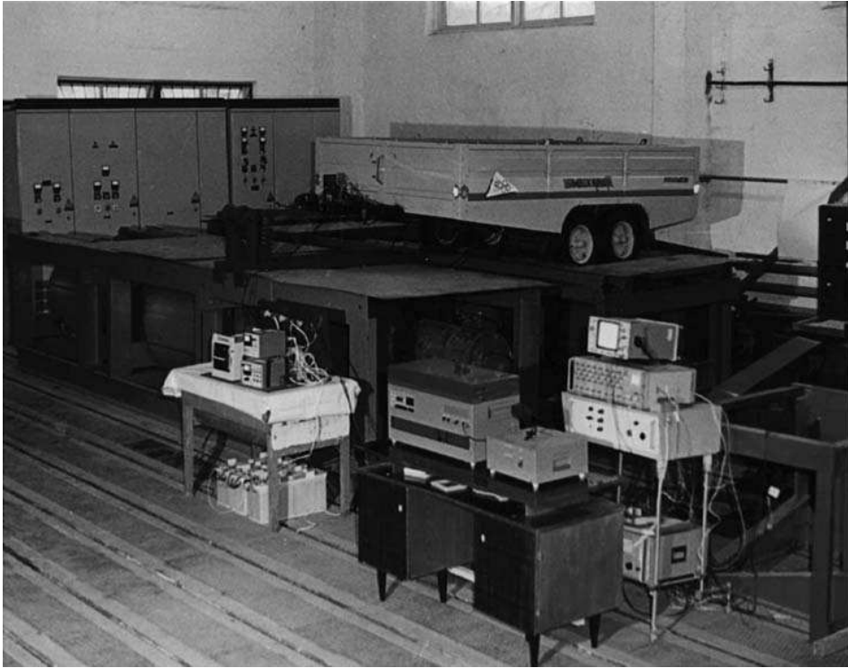
Figure 2.40 Vibration computer controlled equipment with test subject – a car trailer.
