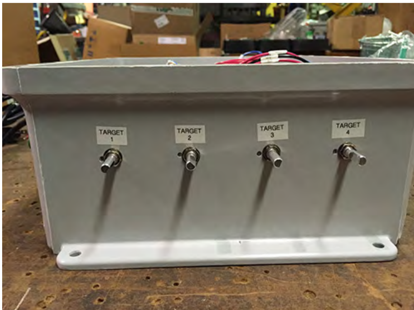
Figure 8F: Target potentiometers adjust for the loudest output volume.
