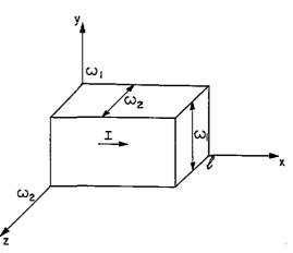
**Figure 5.** A wire of rectangular cross section with sides  $\omega_1$  and  $\omega_2$ , length  $\ell$  and uniform current flow *I*.
