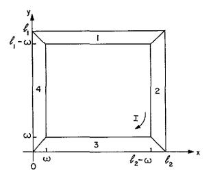
**Figure 1.** A rectangular circuit with sides  $\ell_1$  and  $\ell_2$  and a constant thickness *w*. There is a uniform and constant surface current *l* flowing in the circuit. In pieces 1 to 4 the direction of the current is given by, respectively,  $+\hat{x}$ ,  $-\hat{y}$ ,  $-\hat{x}$  and  $+\hat{y}$ . Here  $\hat{x}$  and  $\hat{y}$  are the unit vectors along the *x* and *y* axes, respectively.
