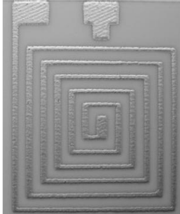
Fig. 3. The screen printed base of 5.5 coils of inductor made on ceramic substrate.
