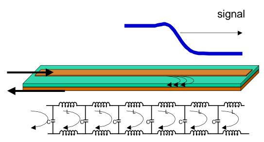
Figure 4 The current at the leading edge of a signal is propagating in a loop that includes the signal path and the return path immediately beneath it.
