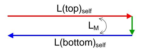
Figure 3. When both wire segments are part of the same loop, the current in the top segment is in the opposite direction as the current in the bottom segment. The field lines from the bottom segment, around the top segment will be in the opposite direction, and subtract from the field lines in the bottom segment.
