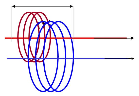
Figure 2 When a second wire carries a current, some of its field lines will completely surround the first wire. These magnetic field lines contribute to the mutual inductance between the conductors.
