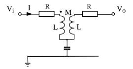
The filter above is to be a band pass filter. There is no load on the output. Where should the second dot be placed - and why?
