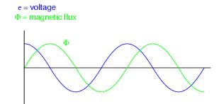
Figure 4: Voltage induced in a coil due to sinusoidally varying flux
