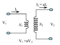
Figure. 12: Ideal transformer equivalent circuit
