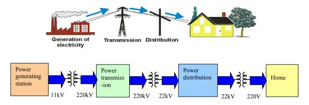
Figure15: Transformers raise/lower voltages in electrical energy distribution
