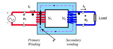
Figure 10: Ideal transformer connected to a load
