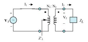
Figure 16: Load impedance as seen by the source
