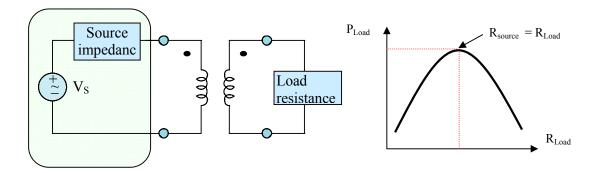
Figure 20: Transformer application for impedance matching
