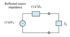
Figure 19: Simplified circuit
