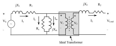
Figure 25: Equivalent circuit of a practical transformer
