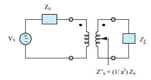
Figure 18: Source impedance as seen by the load
