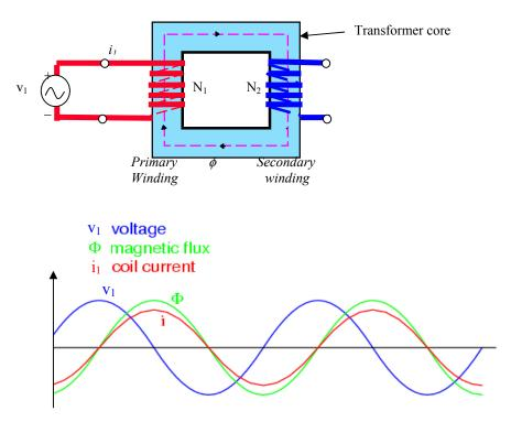
Figure 9: Voltage, current and flux in the primary winding
