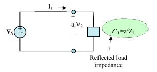
Figure 17: Simplified circuit
