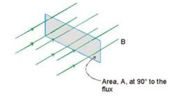
Figure 3: Magnetic flux density
