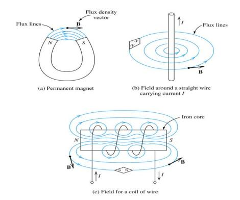
Figure 1: Magnetic field created by (a) permanent magnet, (b) straight wire, (c) coil of wire wound on an iron core
