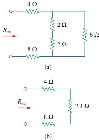
This 4- $\Omega$  resistor is now in parallel with the 6- $\Omega$  resistor in Fig. 2.35(a); their equivalent resistance is
