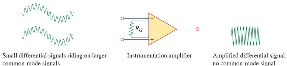
**Figure 5.39** The IA rejects common voltages but amplifies small signal voltages. Floyd, Thomas, L, *Electronic Devices*, 4th edition, © 1995, p. 795. Reprinted by permission of Pearson Education, Inc., Upper Saddle River, NJ.
