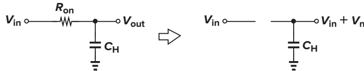
Figure 13.24 Thermal noise in a sampling circuit.
