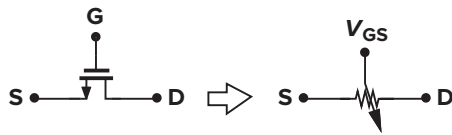
Figure 2.13 MOSFET as a controlled linear resistor.
