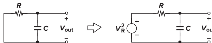
Figure 7.15 Noise generated in a low-pass filter.
