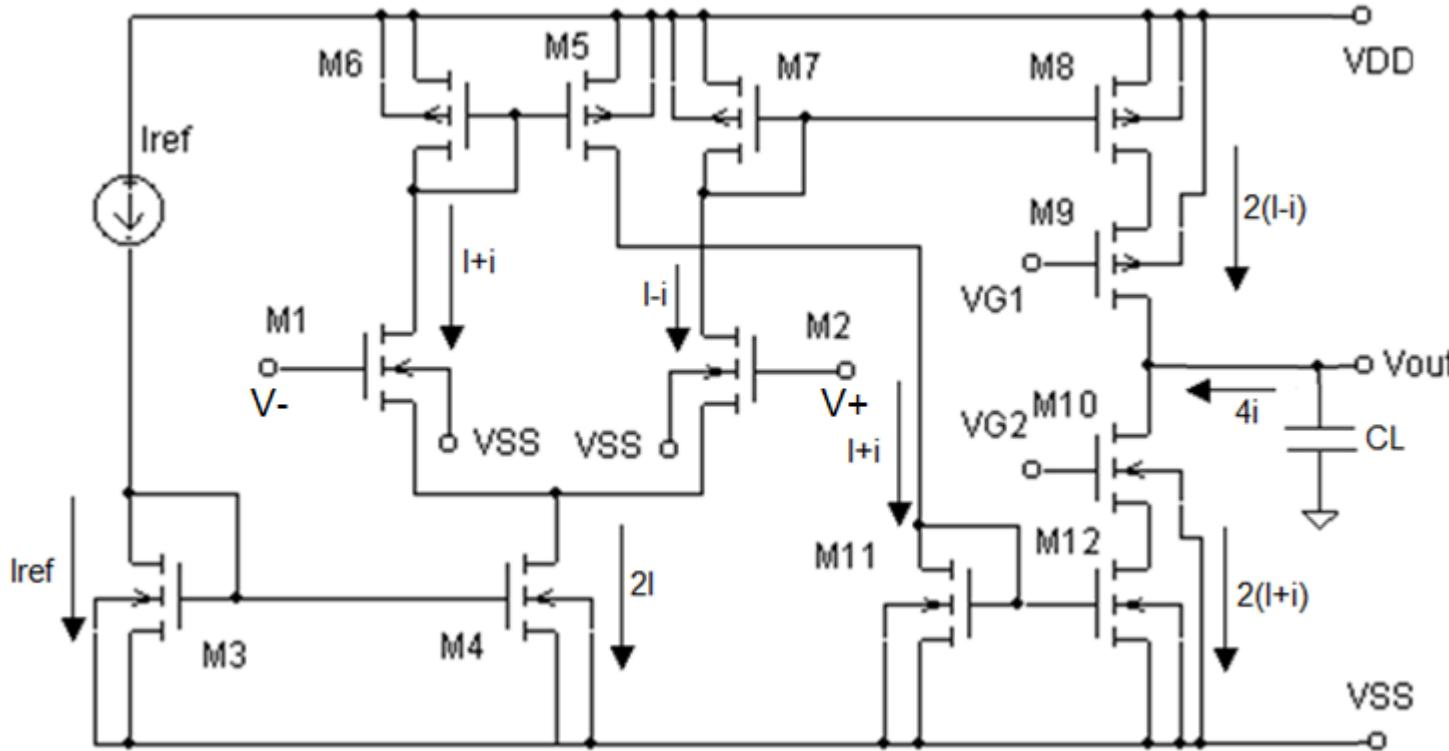
$$I_{ref} = 20\mu A; I = 10\mu A; I_D = \frac{k}{2} \frac{W}{L} (U_{eff})^2; U_{effn} = 0,1V; U_{effp} = -0,1V$$
