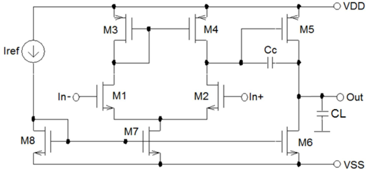
$$BW = f_{pd} = \frac{g_{dsp4} + g_{dsn2}}{2\pi(A_{ud2} + 1)C_c} \quad f_{nd} \approx \frac{g_{mp5}}{2\pi C_L} \quad f_z = \frac{g_{mp5}}{2\pi C_c} \quad (\text{положителна нула!})$$
