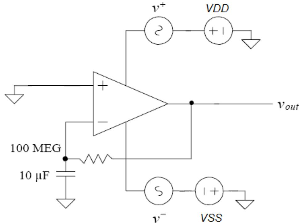
$$\text{PSRR}^+ = \frac{A_u}{v_{out}/v^+}; \quad \text{PSRR}^- = \frac{A_u}{v_{out}/v^-}.$$
