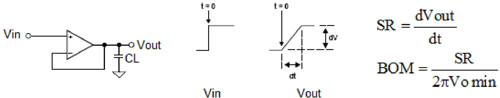
$$SR = \frac{dv_{out}}{dt} = \frac{\Delta v_{out}}{\Delta t} = \frac{I}{C_L}$$
