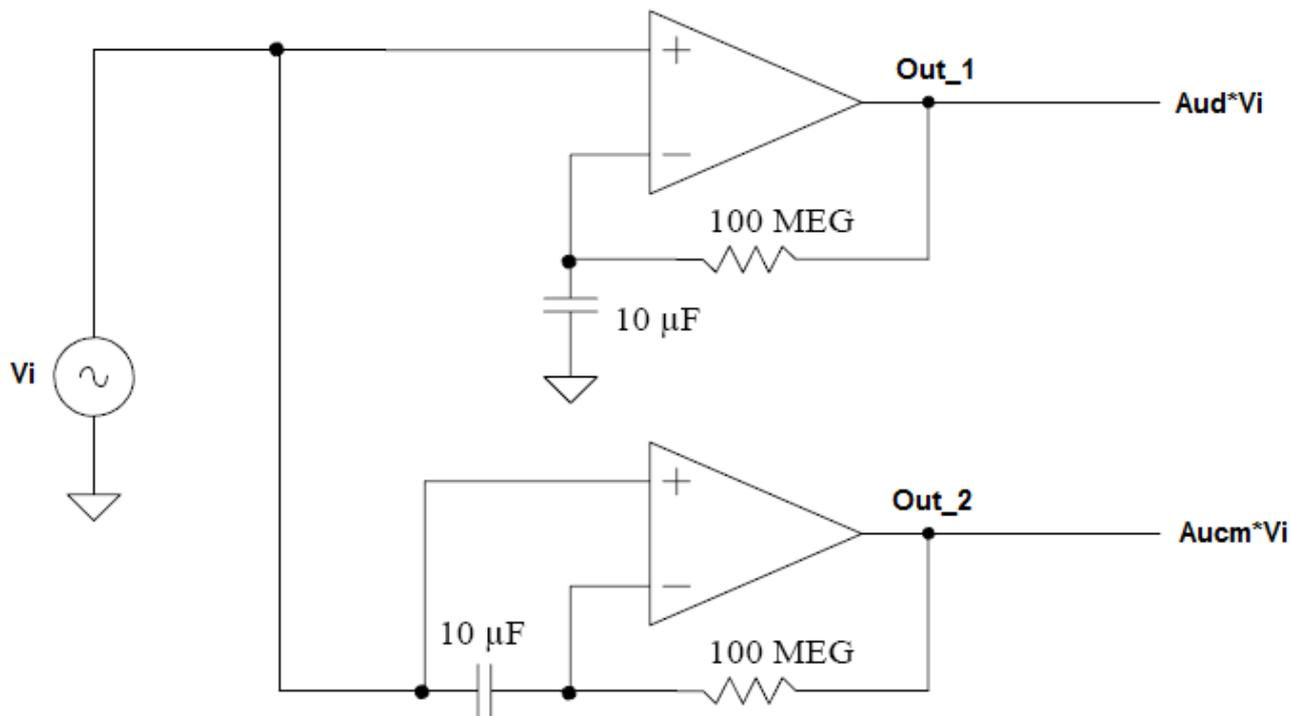
$$\text{CMRR} = 20 \log \left( \frac{A_{ud}}{A_{ucm}} \right) = 20 \log \left( \frac{V(\text{Out}_1)}{V(\text{Out}_2)} \right)$$
