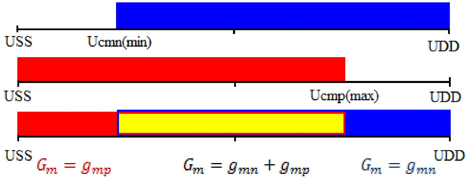
$$U_{SS} \leq U_{cm} \leq U_{cmin(min)} \rightarrow G_m = g_{mp}; \quad U_{cmp(max)} < U_{cm} < U_{DD} \rightarrow G_m = g_{mn};$$
